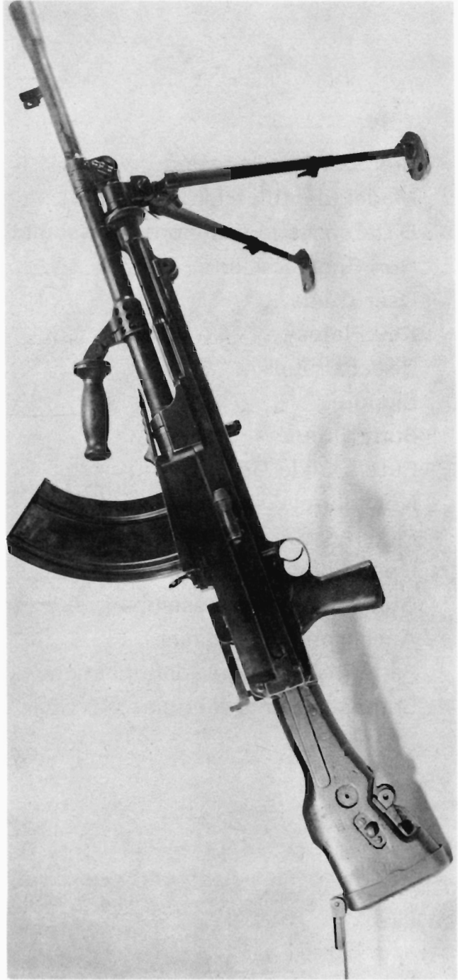
.303-in. ZGB 1933 (Model No. 2) Trials Light Machine Gun. Note the finned barrel with "muzzle brake" holes for the flash hider, position of the rearsight and its drum and the butt monopod. M.O.D. Pattern Room.
