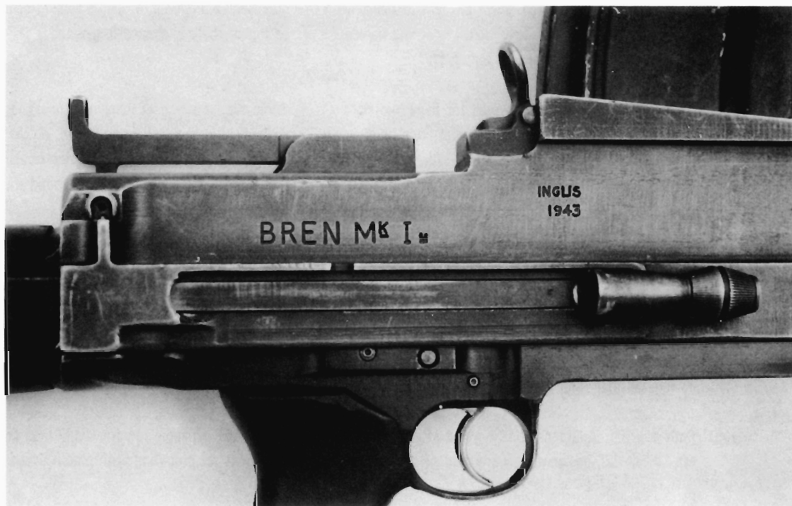
Inglis Bren Mk I(M) body marks. Note Mk 1 backsight, Mk 1 cocking handle & recessed Mk 1 mag catch. J. Watter.
