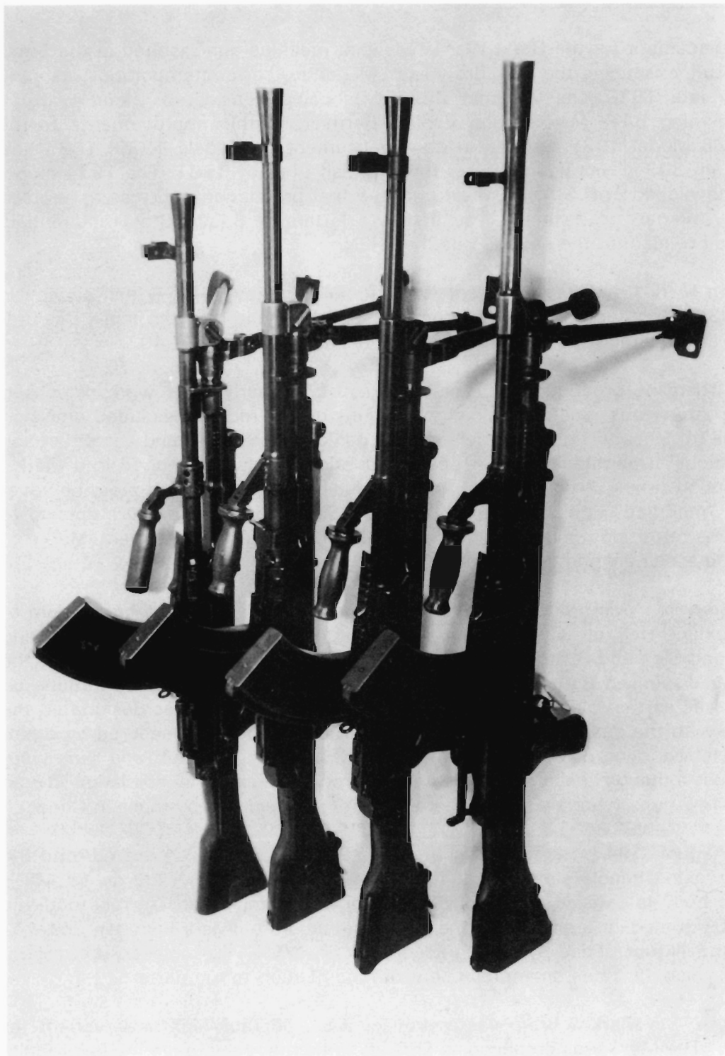
Different Marks of the .303 Bren L.M.G. From the bottom—Guns Mark 1, Mark 2, Mark 3 and Mark 4. Although particular body details are indistinct, the various barrel, bipod and butt configurations are shown. Note the different lengths and sight fixtures of the barrels (Marks 1*, 2, 2 and 4), the different carry handles, and various butt shapes. M.O.D. Pattern Room, Nottingham.
