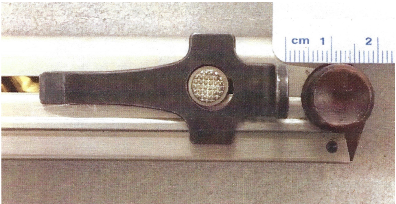
53.5 mm Long Neck magazine loading tool (Schraubenzieher) in position with 8 cartridges in the magazine and no downward pressure showing additional space available. See paragraphs 2 and 4 above.
