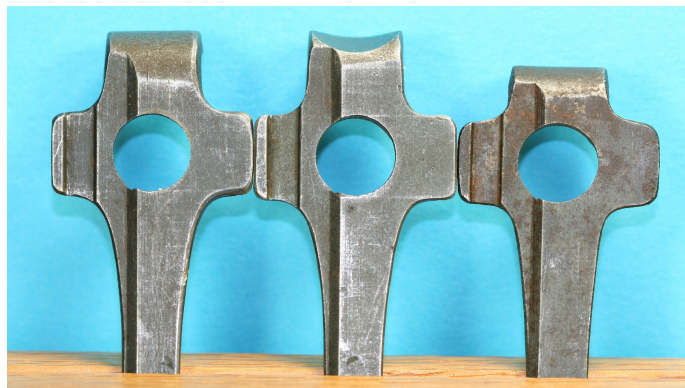
A non-modified and a modified long neck magazine loading tool neck length compared to a 1904-sized loading tool.
