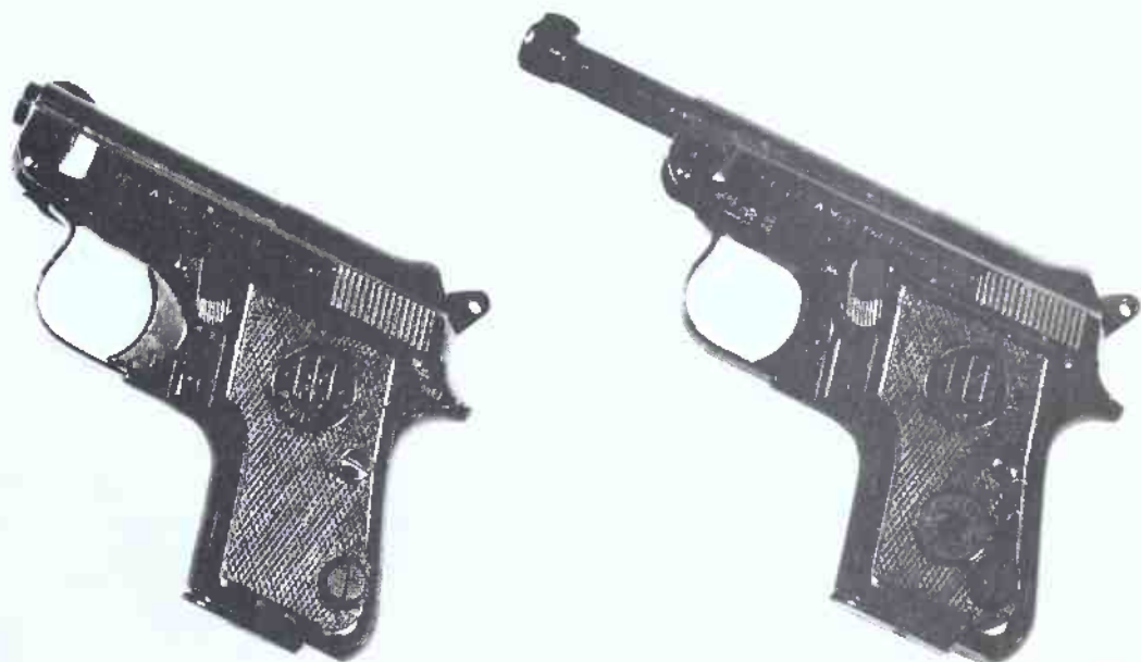
Beretta Model 950 and Model 950 special. These weapons are identical except for the barrel length. Notice the slide markings on the longer barrelled 950 giving its American name 'Minx' (Pattern Room, Enfield)
