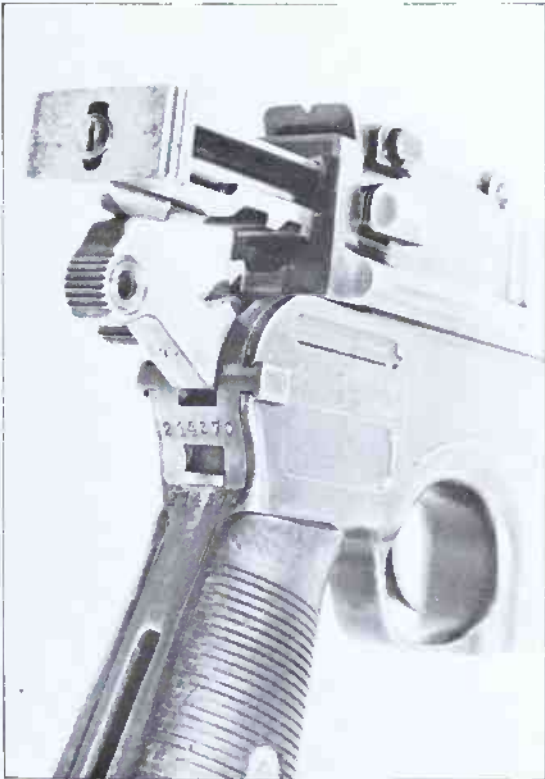
The Bolt shown to the rear. Notice the locking lugs Author's Collection
