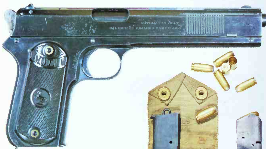
A Colt .38 Automatic Model 1900. Notice the 1902 type rounded hammer
