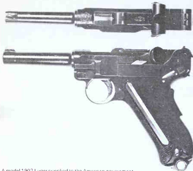
A model 1902 Luger supplied to the American government with the Powel cartridge counter (R. Shattuck) Right: The Powel cartridge counter
