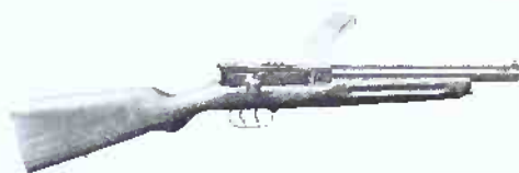
An F.N. 1935 Submachine gun with a toggle action (F.N.)
