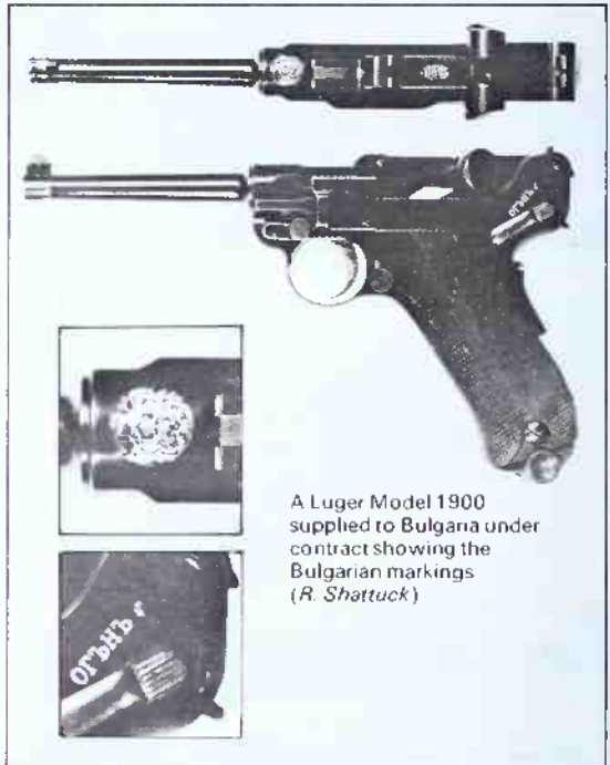
The toggle at the top is from the Seven Shot and the bottom is standard ( R. Shattuck )
