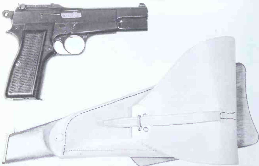
Late production tangent sighted Hi Power with flat wood stock and attached holster. Bowman .
