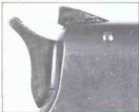
Colt Model 1900 sight safety shown in raised position (Major Borthwick)
