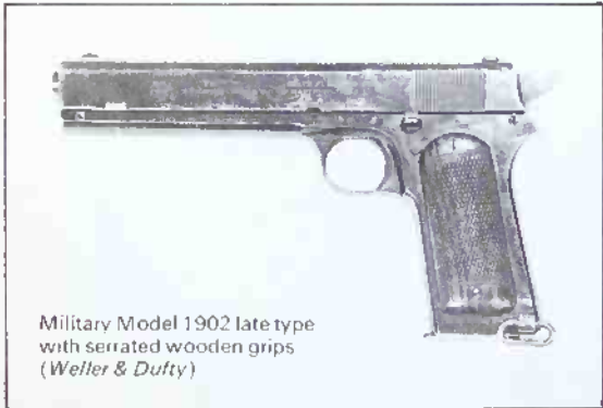
Military Model 1902 showing the spur hammer and the finger grips at the rear of the slide
