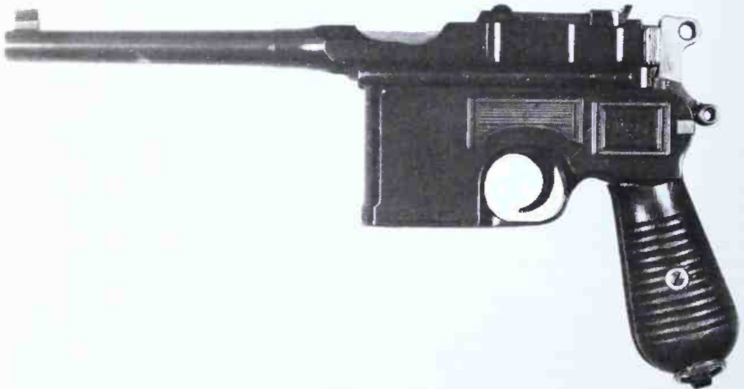
A late type post-war Commercial. Notice the lack of milling on the rail below the barrel extension compared to that of the early type ( Pattern Room, Enfield )
