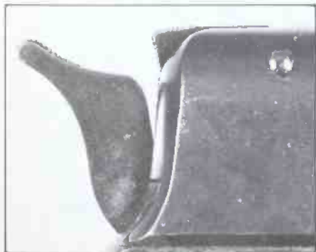
Colt Model 1900 sight safety in safe position (Major Borthwick)
