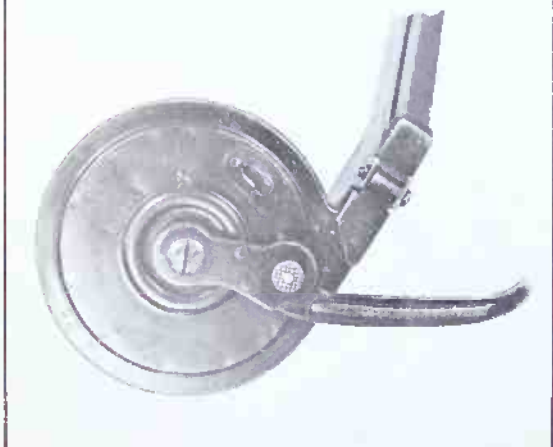
The latter type of Snail Drum Magazine showing the loading lever in the open and closed positions (Lowland Brigade Depot)
