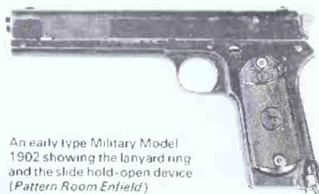
Colt Military Model 1902 early version with the rounded hammer and checkered slide grip (Pattern Room Enfield)
