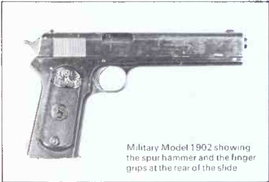
Right side of Colt Military Model 1902 with the 1908 modifications (Pattern Room Enfield)
