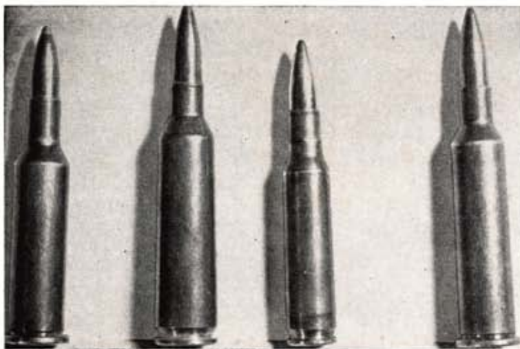
Most popular bench rest loads currently are (l. to r.) .219 Don, 22-250, .222 Remington and .219 Improved Zipper.
