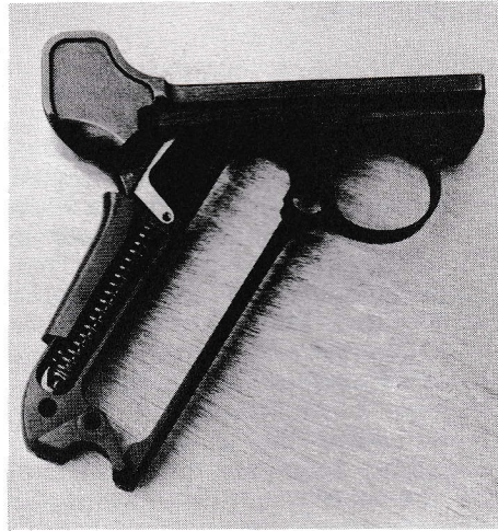
Long Swiss grip safety wraps around and disappears under stocks on right side. Mauser will do likewise, but will shorten safety for an O6-ish look.
