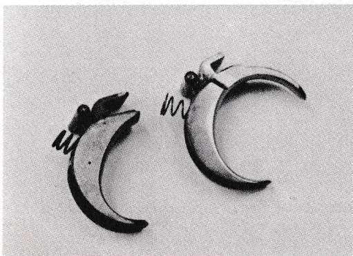
Wraparound 06 trigger with machined-on mounting pin was ridiculously expensive. Though they nose-bobbed it, the Swiss couldn't make it much cheaper. Mauser will prudently cast this part.
