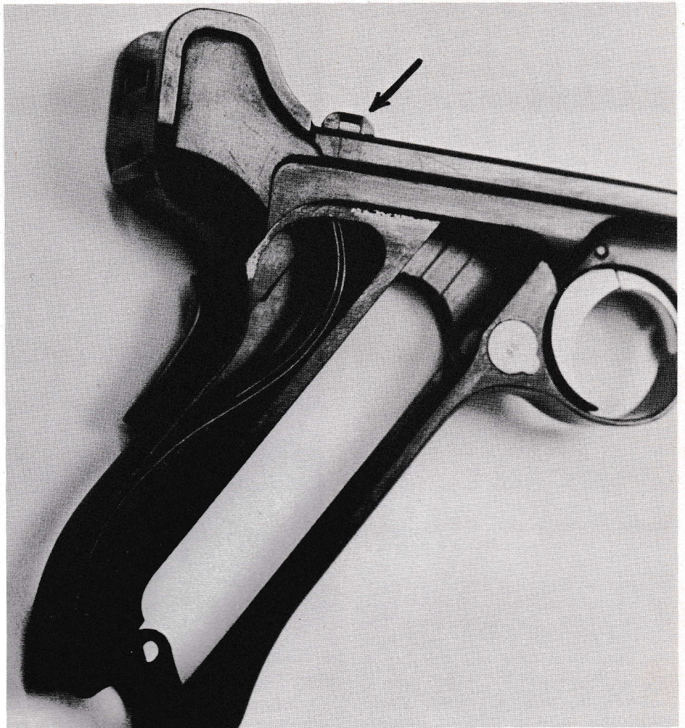
1900-1904 models had 2-piece laminated recoil spring — a poor arrangement indeed. Toggle-lock hook (arrow) was dovetailed into frame.
