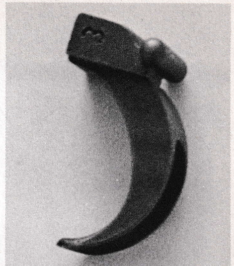
Sideplate and trigger from #1 9mm prototype shows how it looks when it comes out of the wash — it looks pure Swiss. Cast trigger will still take a worthy bit of machining to bring it to shape. Mounting pin diameter must be reduced, trigger bar engagement slot cut, and trigger spring mounting hole drilled. Then we polish, blue, and hand fit, not to count inspections. The Luger still costs money to build.
