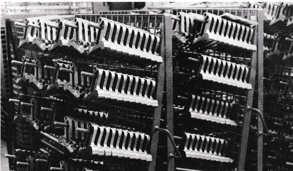
Mauser let an immediate order for 30,000 frame forgings to the smithy, had some 5,000 of these in work when Stevenson made these photos in late March. Later orders will level off at 1000 a month.
