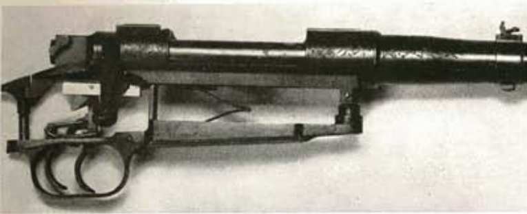
Pilot model of original Newton action had small bolt knob typical of old rifles, and regular set triggers of foreign style.
