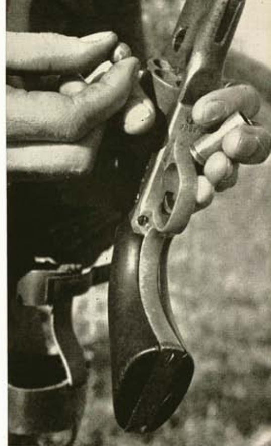
Round bullets for mid-range accuracy are put one at a time on chambers.
