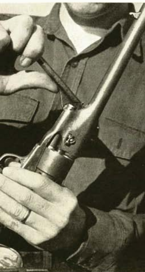
Compound loading lever is used to press each bullet down into chamber.
