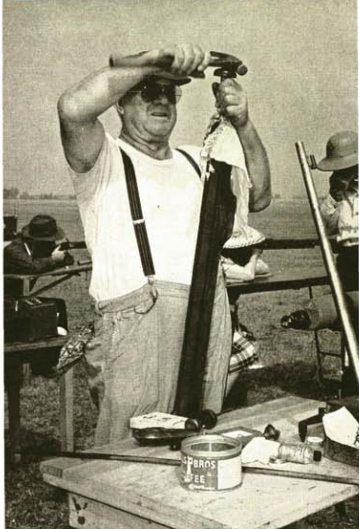
Bench rest rifle is loaded by Ralph Dunn of Fort Wayne, Ind., by hammering cloth-patched bullet into bore.
