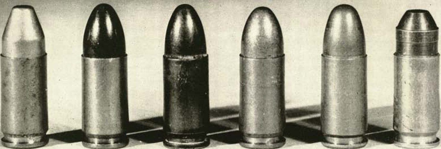
Bullet shapes of 9mm progress from first Luger load (left) through tommy gun rounds to Army test .35 cal. (right).
