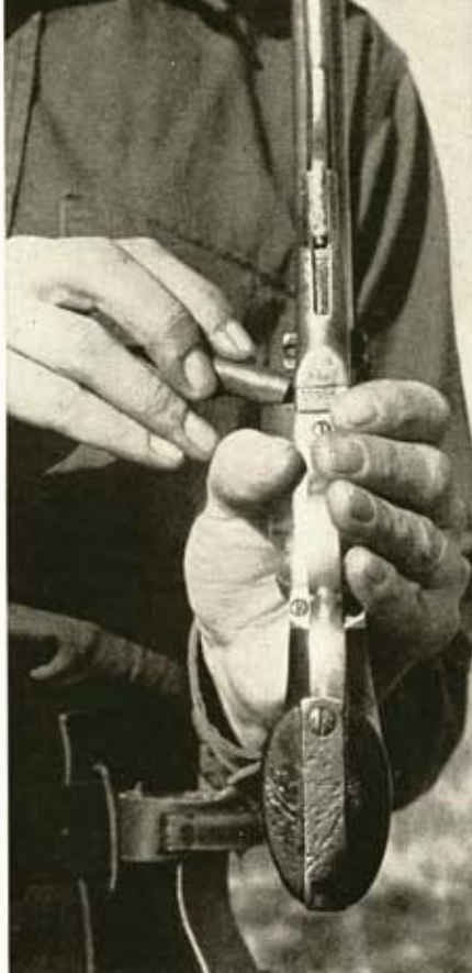
Measured charge is poured into each chamber with hammer on half-cock.
