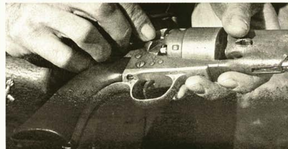
Colt frame has capping cut-out so percussion caps may easily be placed onto chamber cones or nipples. Cyclinder spins free for loading at half-cock.
