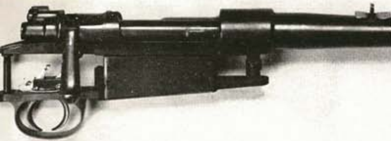
Newton's Special fore-and-aft set triggers on .256 rifle was fitted on Mausers after his first company failed.
