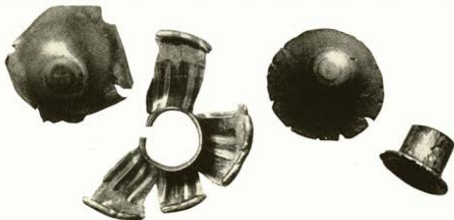
German service 9mm bullet shed its jacket (left) in penetrating \frac{1}{8} " steel plate but .45 slug burst jacket, flattened out and stopped cold (right) on steel.
