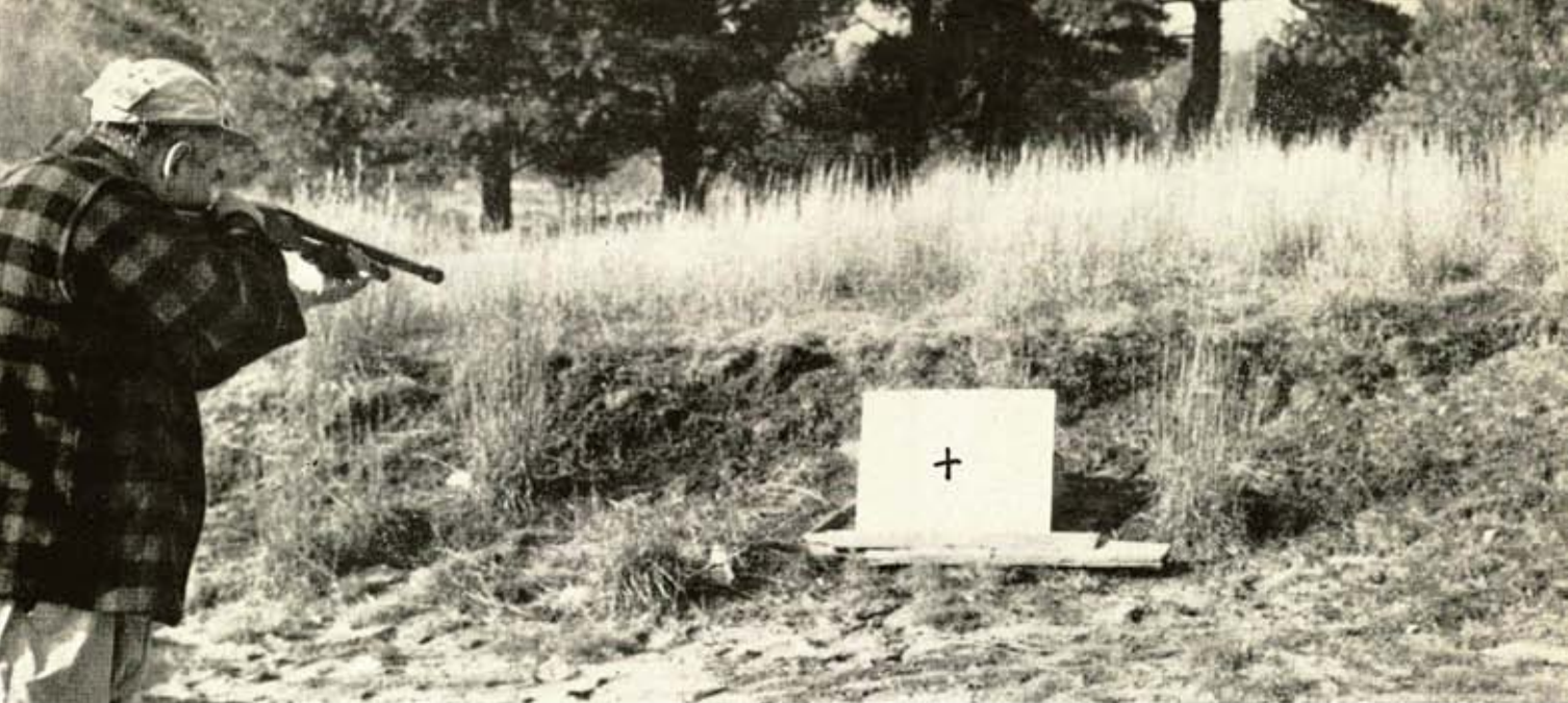
Master-choke equipped shotgun is fired by Charles Bliss at target paper set up only ten yards off to check pattern. New patterning method would actually permit shooter to test his shotgun in basement, if he had adequate backstop.
