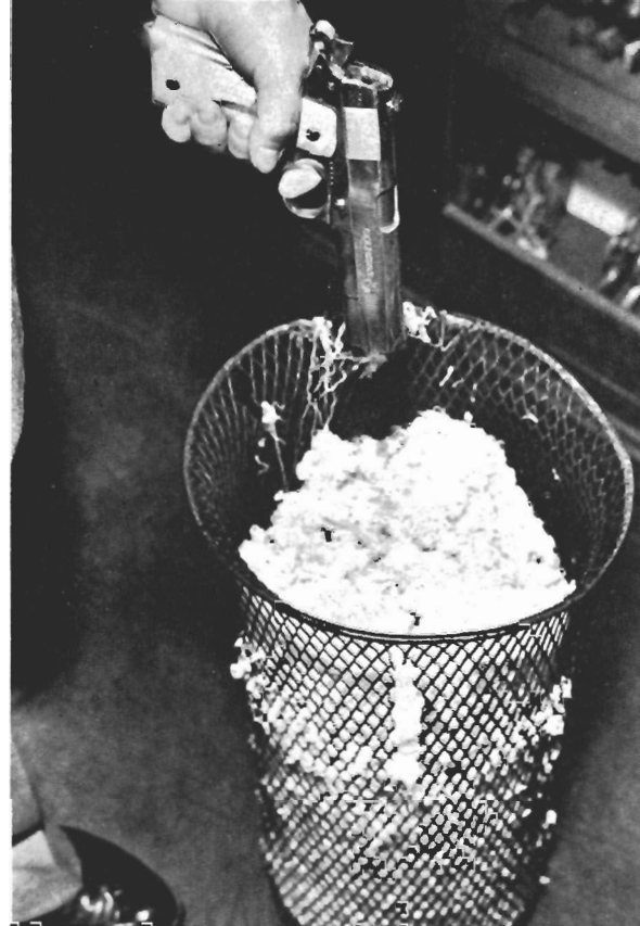
Test bullet from evidence Colt .45 is fired into basket of cotton waste at Chicago crime laboratory to get bullet undamaged.
