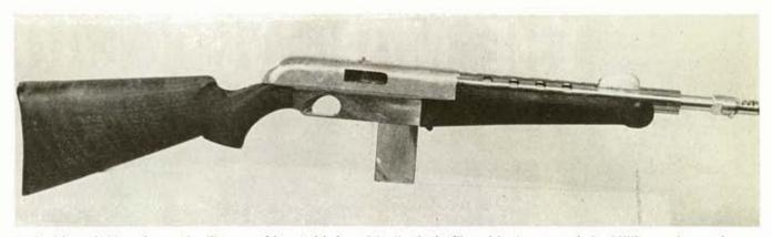
Locked-breech blow forward military carbine (with barrel in "unlocked" position) was made by Hillberg when ordnance engineer with aircraft firm in World War II, used style curves which were later dominant in Whitney pistol.
