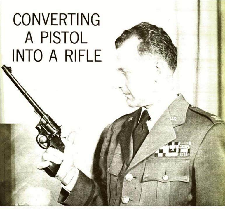
Colonel Ward Betz fitted piece of .30-30 rifle barrel to his old New Service Colt in wildcat revolver cartridge experiment which resulted in .30/357 bottleneck handgun pill having many shooting qualities of a rifle load.
