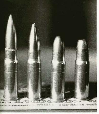
Betz-Lindahl .30/357 wildcat was made by necking .357 revolver cases to "rifle cartridge" shape and loading with 150 grain, 110, 93 and 86 grain cast bullets.
