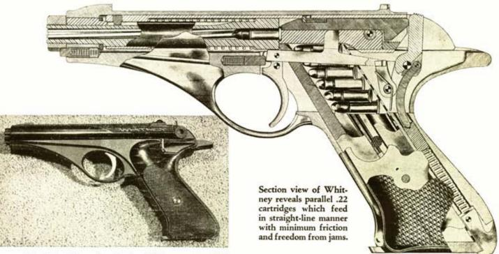
Futuristic styling of production Whitney automatic is enhanced by two-tone black anodizing finish. Thumb safety is fast, snaps off by thumb pressure upwards.
