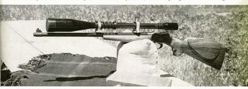
Springfield barrel on small Martini action did not stabilize longer bullets at moderate velocities obtained, but 150 grain M2 slug did fairly well, 3" at 100 yards. Unertl 12X scope was employed during testing from sand bag rest.
