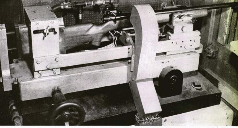
To prevent human error from entering into accuracy tests and invalidating results, machine rest was used to rigidly hold Winchester (above) and Remington rifles during thorough study of .22 cartridges on windless indoor 100-yard range.
