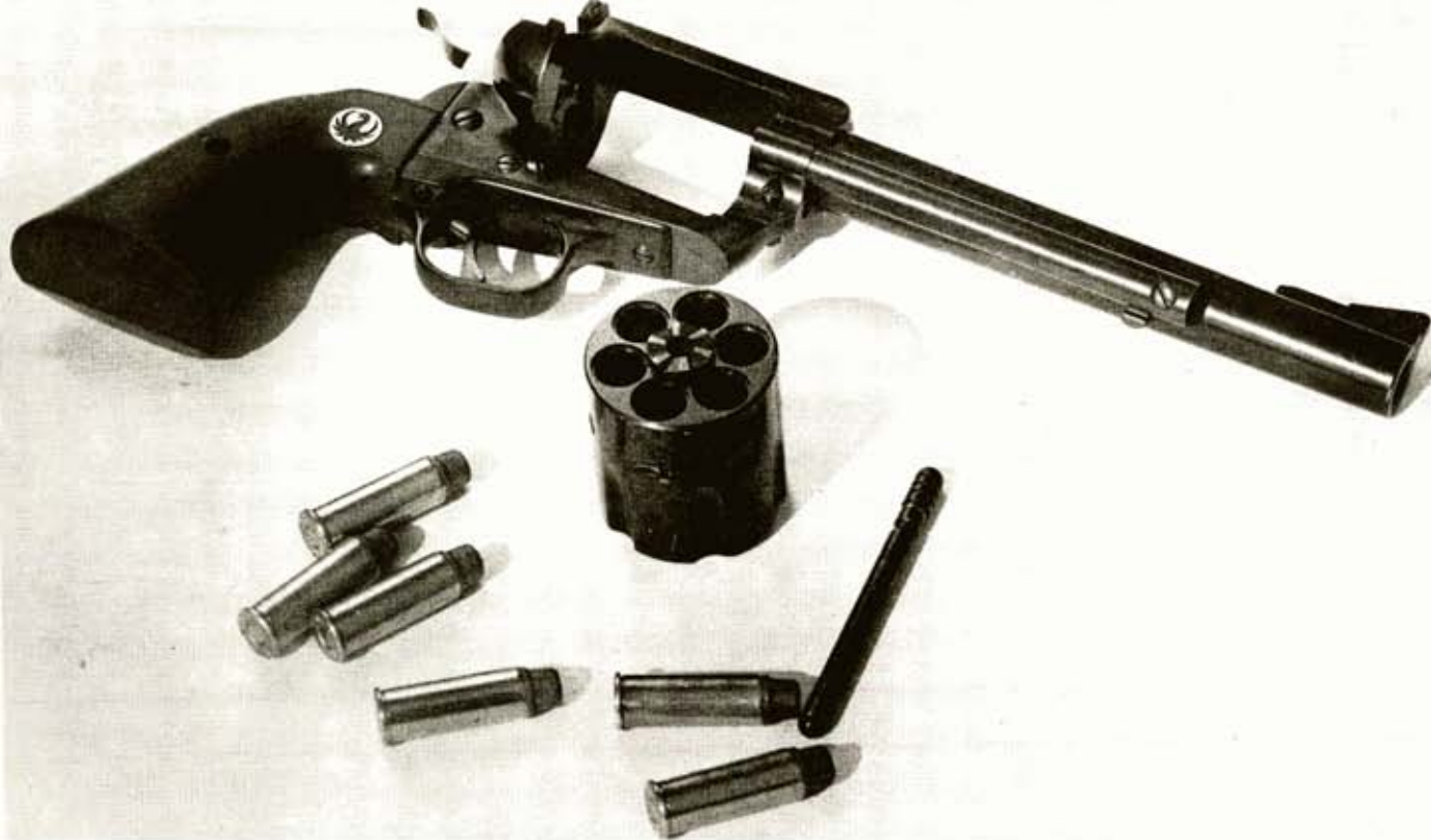
Simple take-down of single action revolver where cylinder drops out when pin is pulled has much to do with present demand for the type. Rugged strength important to frontiersman in a handgun is still needed in knockabout camping service.
