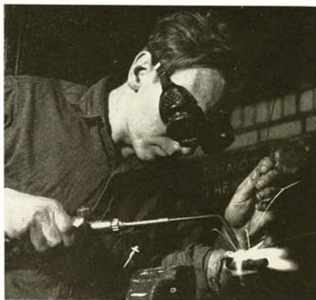
Water-soaked rags protect locking lugs, and goggles protect workman's eyes, as student welds bolt handle.
