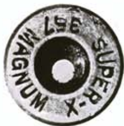
Primer holes off-center result in inaccuracy.
