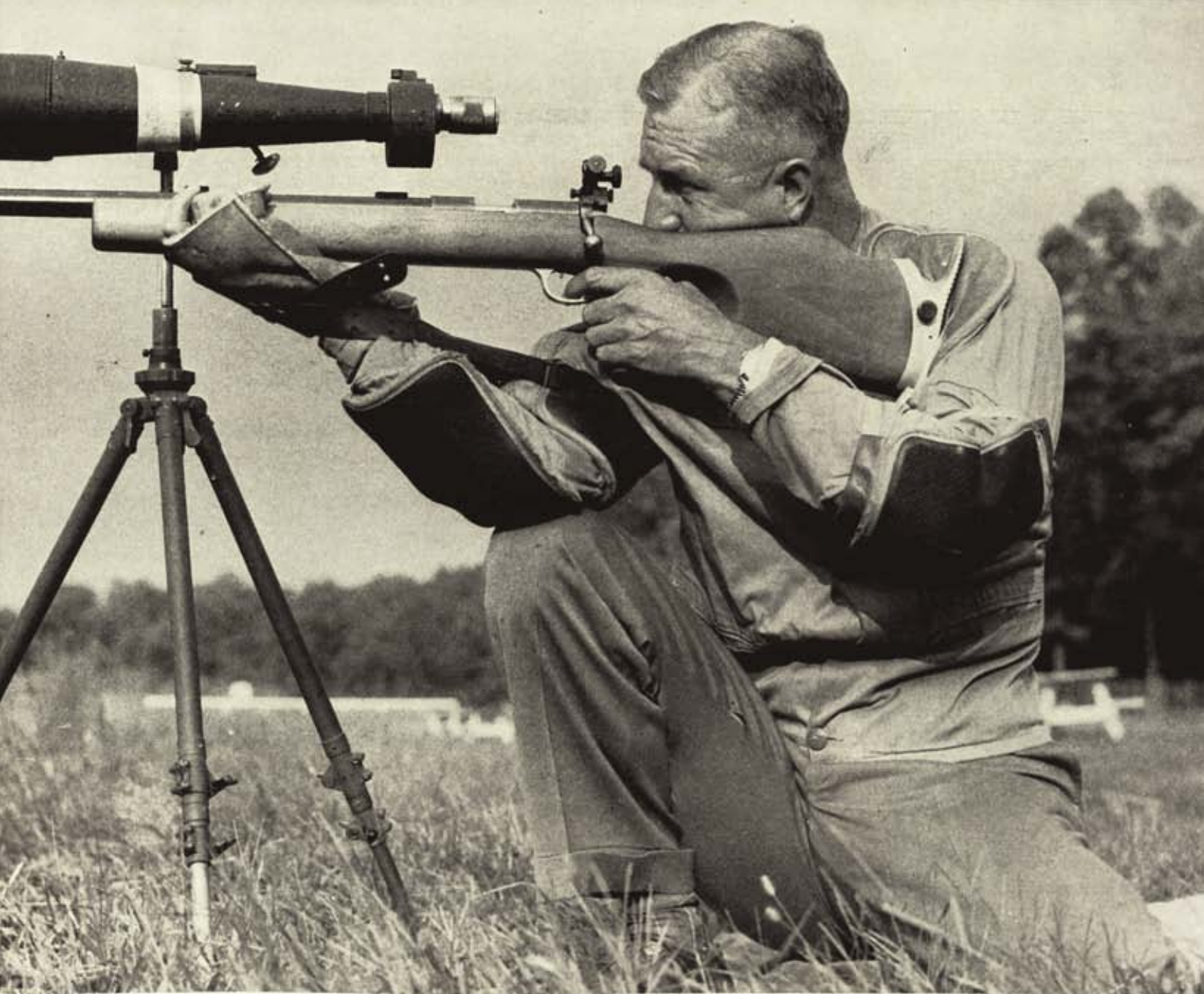
Shooting custom-made left-handed Dunlap rifle as "control," Larry Moore aims at target in tests of low-priced rifles. Dunlap has receiver and bolt similar to M52 Winchester, Canjar trigger, Eric Johnson barrel and thumb-hole stock.
