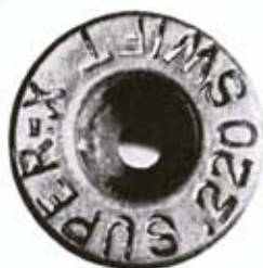
Primer holes off-center result in inaccuracy.
