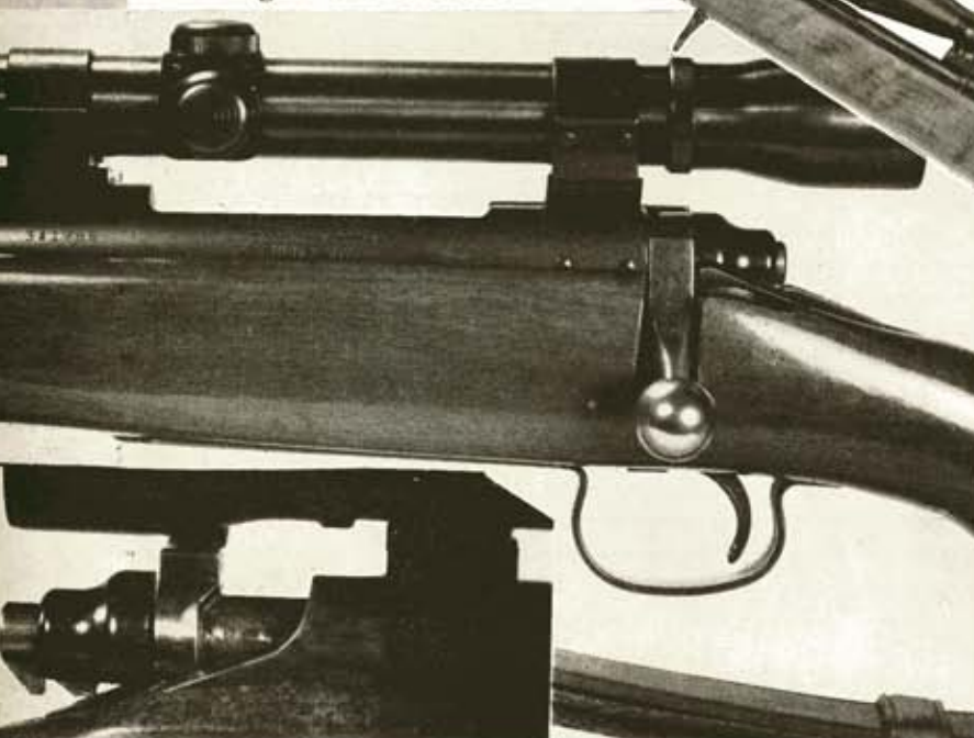
Left-hand rifle altered by Dale Guise (below) has breech welded and primary extracting is cam reversed.
