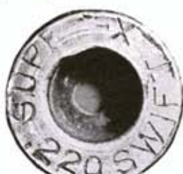
Soft brass in case head makes extraction hard.
