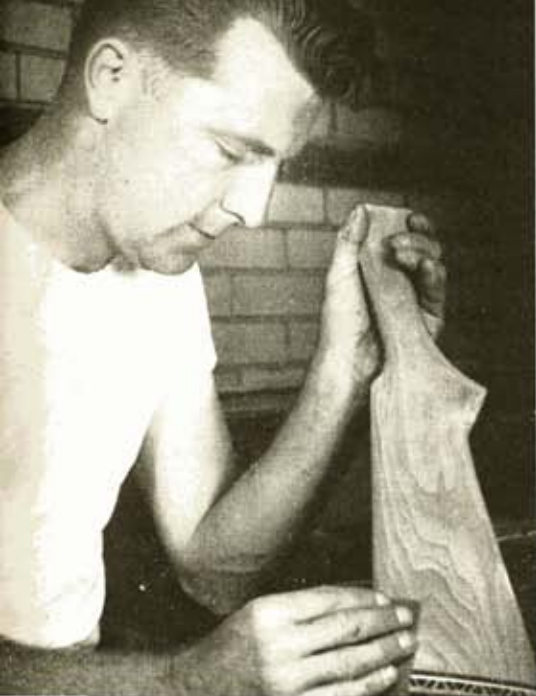
Randy Atchison applies final grit-paper rubdown to well-grained stock.
