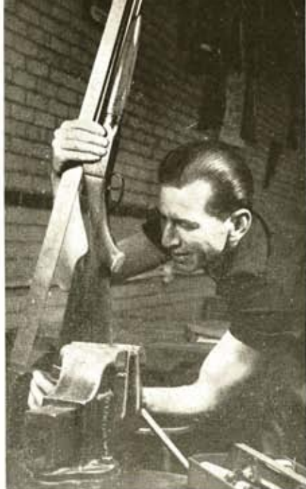
Drop measurement on fine custom-stocked Ithaca double gun is checked.
