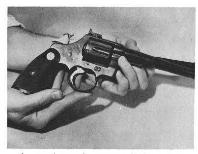
volvers, permits strength, accuracy combined with easy loading and unloading. Not as fast as S&W top-break, it is better for shooting hot loads.
