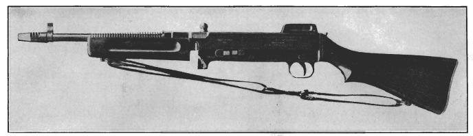
English experimental Thompson Sub-Machine Gun made in 9mm Parabellum caliber by BSA Co.
