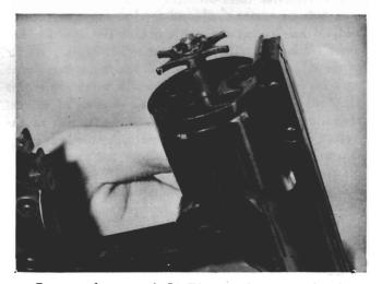
Pop-out feature of S&W auto-ejecter top-break revolvers threw empty shells clear of frame but might eject loaded shells by accident.
