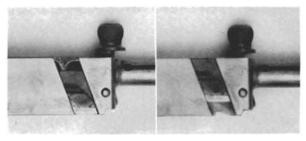
Slide, block and lock in "locked" and "unlocked" positions.
