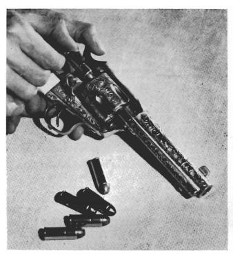
Loading of Frontier was very slow but in 1873, contrasted with older cap-and-ball models, it proved satisfactory. Shells are loaded singly.
