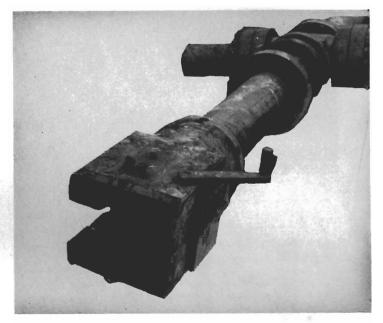
Breech block of HDP gun is similar to ordinary Krupp sliding breech. The bolted flange design permitted easy repair in field after accidents.
