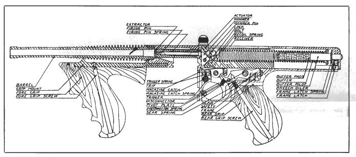
Plan view diagram through center line of regular Model 1921 Tommy Gun in .45 caliber.
