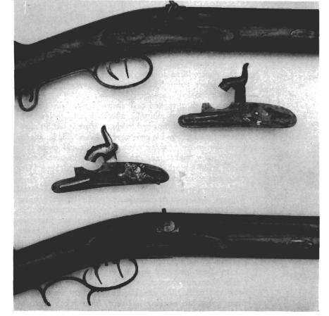
Inside top Hawken lock is stamped maker's marks. Only "John", "M", and "C1717" remains, bolster cut-out having removed other stamping. Locks by Golcher are known and Hawken workman John Gemmer fitted them. Barrel of top gun is attached by "Carbine-like" patent breech.
