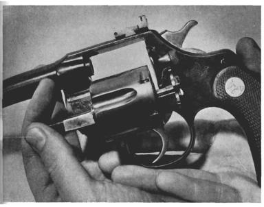
Swing out simultaneous ejection feature of solid frame construction of modern Colt ("customized" Official Police .38 shown) or other top-quality re-
