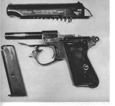
Pulling down trigger guard at front, then pulling slide to rear and upward is procedure for take-down. Be sure gun is empty and magazine is removed.
