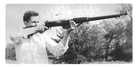
Top: bolt of PC Thompson rifle has already slammed shut but fired case is still in air, illustrating slowness of operation, easy ejection. Below: bolt may be just discerned lifting out of frame recess, as case sets back in dry chamber. Gun shot well with oiled cartridges or dry ones; had very easy kick.
