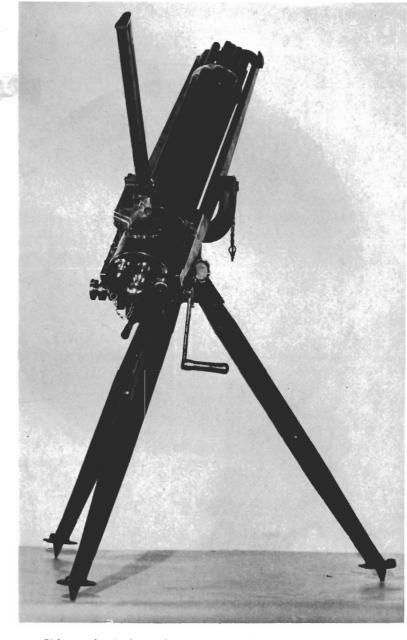
Side-crank Gatling shows massive breech housing, polished steel trunnion arms with sights attached.
