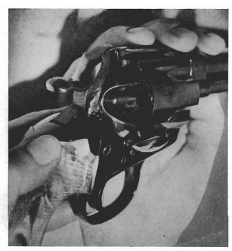
Side ejection (shown on Bisley model variation) permitted rigidity of solid frame construction and avoided accidental dropping of loaded shells.
