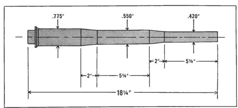
Dimensions of diagram show small size to which the test barrel was safely thinned. Allowing a good margin with known barrel steels gives . . .
