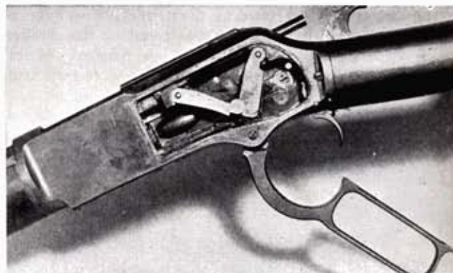
Middle joint of Winchester 76's toggle lock is collapsed by moving finger lever forward, draws bolt back.
