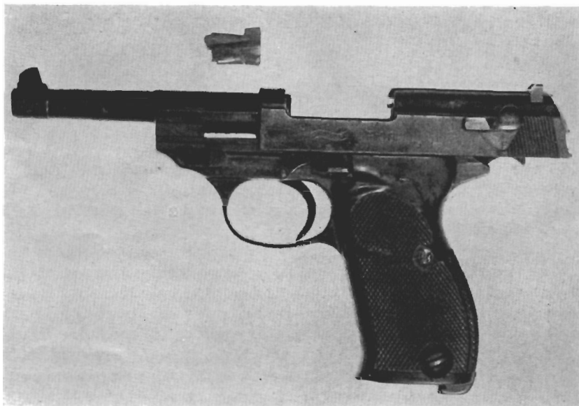
Reassembling P-38 auto pistol without its essential locking block (small piece separate) will result in severe damage, may be blowing off slide.
