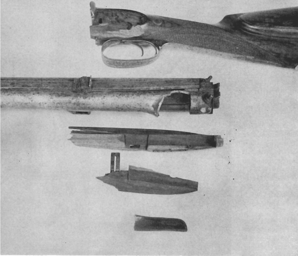
Fine English percussion double-gun was destroyed by deliberate ignorance on the part of the shooter when he loaded Damascus barrels with modern nitro powder charge "just to see what it would do." He saw.
