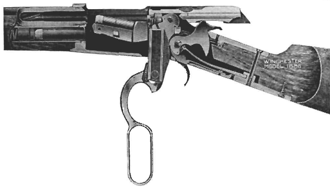
Early classic lever gun was John Browning's slick M86. New Model 88 beats this one for speed and smoothness, and unlike the M86, new M88 has trigger in the lever.
