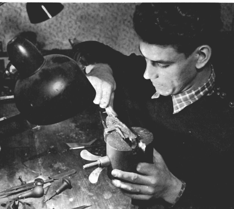
Ball vise holds breech with lock plates fitted as skilled Ferlach engraver works out intricate pattern.
