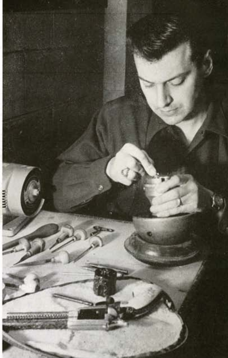
Working on rifle floorplate held on ball vise, author holds edging tool to clean up the first chased lines of pattern. Grinder is near to keep the tools sharp.
