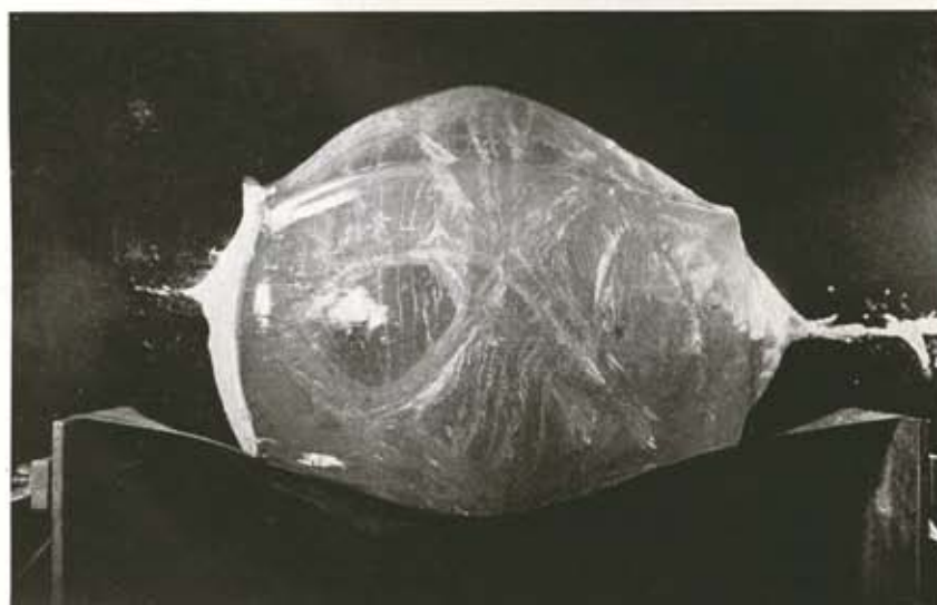
Caliber .30 150-grain Silver-tip bullet passing through 5" square gelatin expands block like meat of animal, although bullet has left target.
