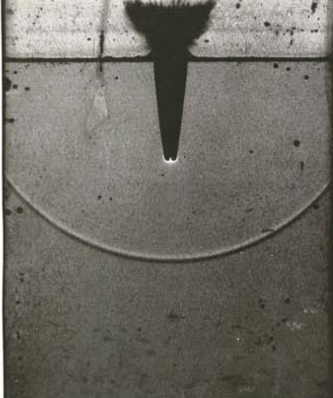
Curving shock wave in water, as in tissue, moves at the speed of sound ahead of the slowing steel ball.
