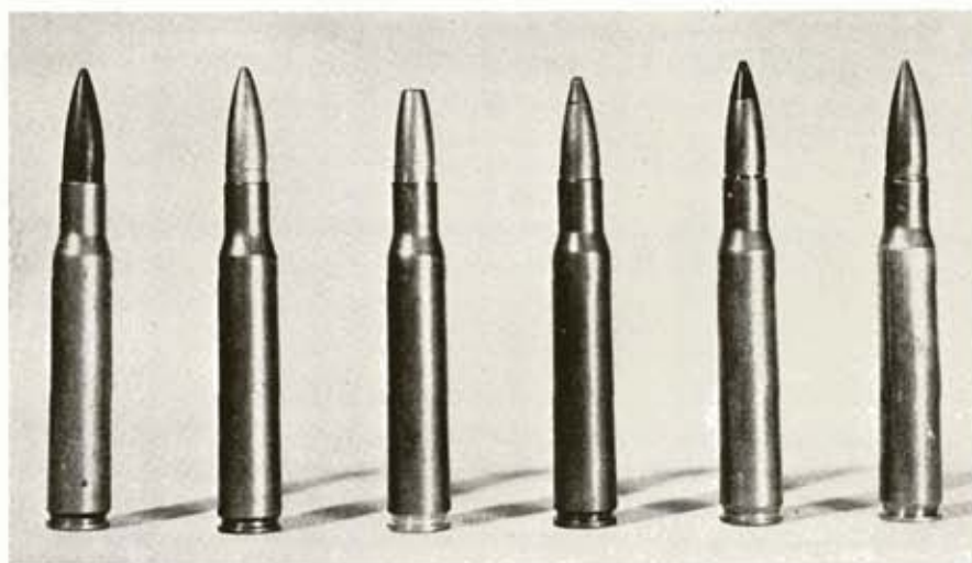
Black M1918 Incendiary (left), M1918 Canadian AP, flat nose M1917 Incendiary, and lead tip M1917 AP are shown with 1945 AP and Ball M2 (right).
