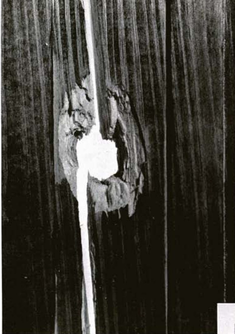
First board was shattered by Magnum .44 in penetration tests, went through seven 1" boards, stopped at eighth.
