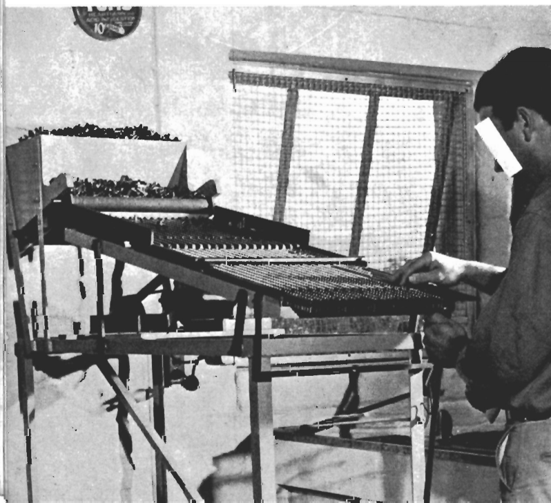
Shell shaker removes all foreign matter from empty cases. Shaker can clean 1500 cases in matter of minutes.
