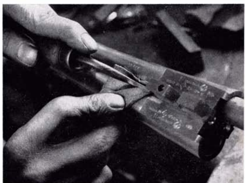
Barrels are polished with emery cloth on point of tool.
