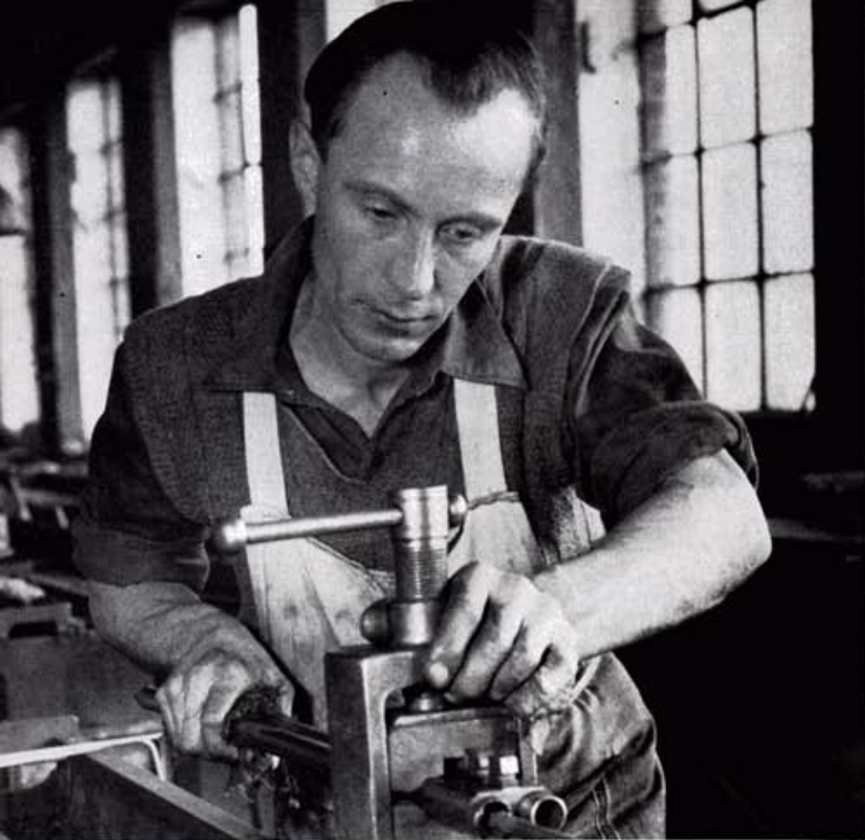
Lapping to smooth bores is done while barrels are held in century-old vise as workman steadies free ends with cotton waste protecting hands.
