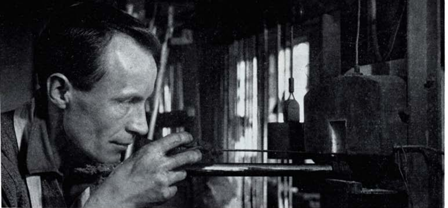
Their muzzles plugged with clay, a set of two barrels is brazed in gas furnace which joins them at breech lumps.
