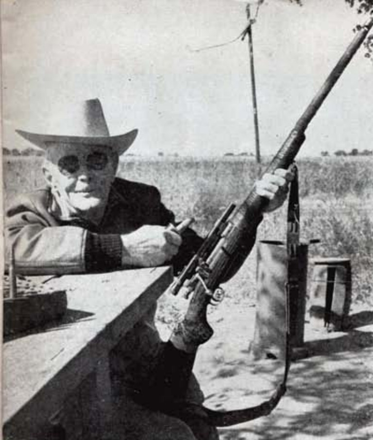
Friction-tape wrapping of Chappel's Springfield sporter minimizes barrel vibrations and contributes to accuracy.
