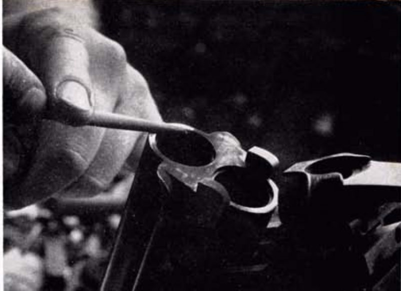
Bright contact spots are filed and breech resmoked to fit.
