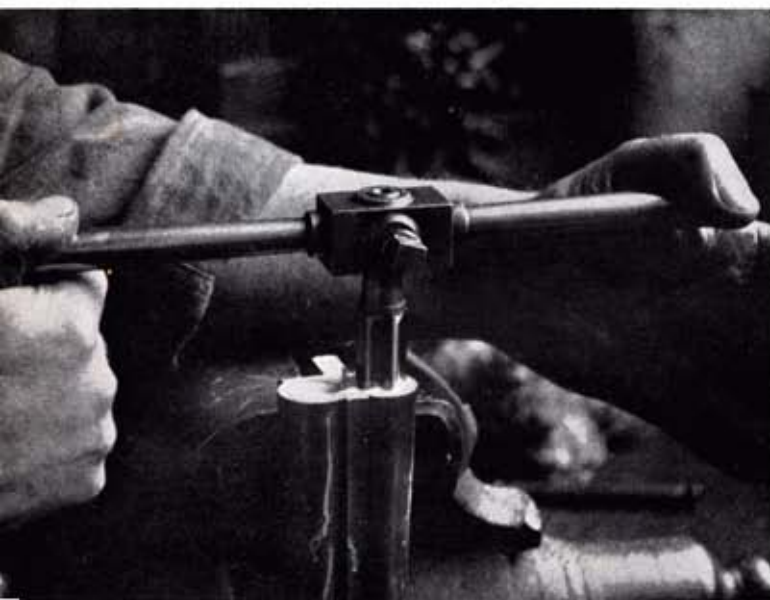
Shotgun chambering is done with rude hand reamer.
