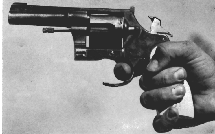
Colt New Service in .357 Magnum makes fine belly gun with guard cut away and sighting rib added.
