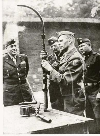
Noted arms writer and expert Phil Sharpe demonstrated captured MP43/1 with 90° barrel to U. S. Ordnance in France. On table is 30° barrel with Zeiss prism sight.
