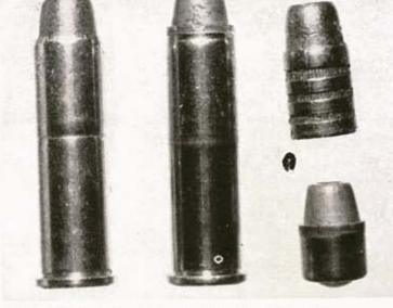
Regular .357 round (left) is loaded with lead bullet, resembles Jugular load (right) with brass gas check.
