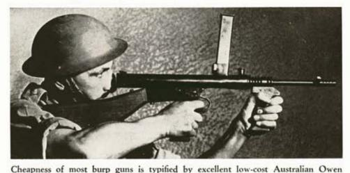
which has quick barrel change and is made of simple tube parts for mass production.
