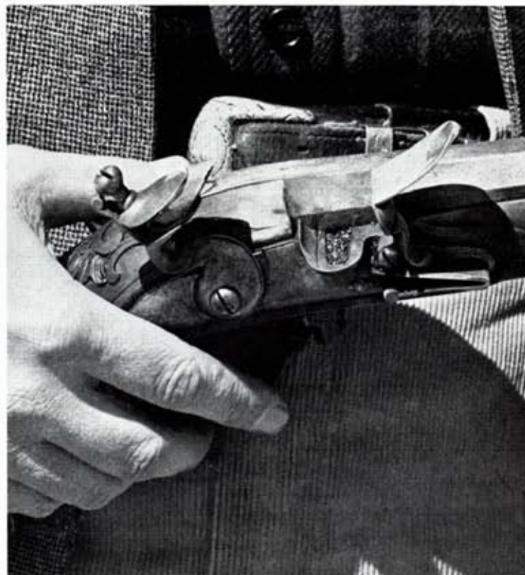
Fine powder is used for priming, then pan cover is closed.
