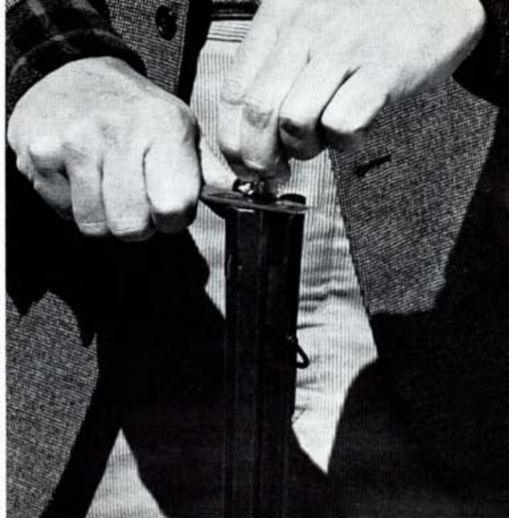
Ball is patched like Kentucky, and patch trimmed by knife.
