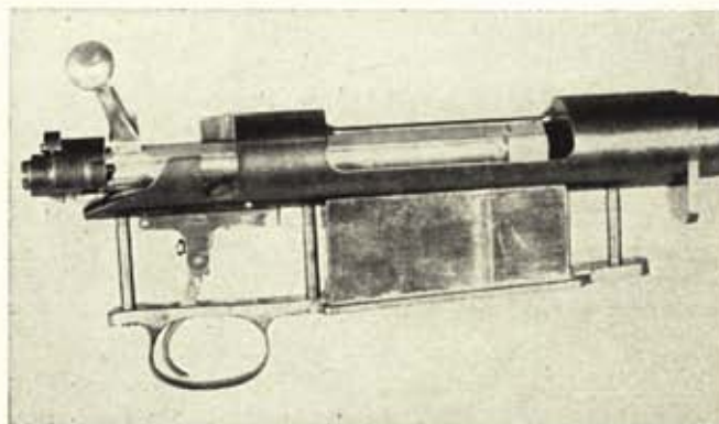
Three-shot repeating action built by Weber for .50 load is 12" long. and fitted with Mauser type box magazine.
