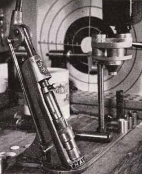
Support bushing prevents shell bulge as wads are seated in Thelson tool.
