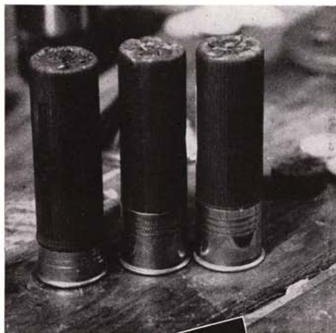
Mistakes in reloading may produce a bulged case which was not loaded in support bushing (left) or too much crimp because shell is short on wads. Third shell at right is loaded and crimped just right for best pattern in author Brandt's Marlin O/U (right).
