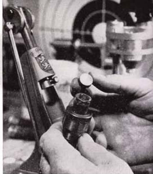
Over-powder and filler wads are next, pushed down while shell is in bushing.
