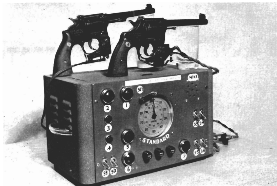
Electric timing equipment of McGivern used on both Colt and Smith & Wesson revolvers gave precise shooting times.
