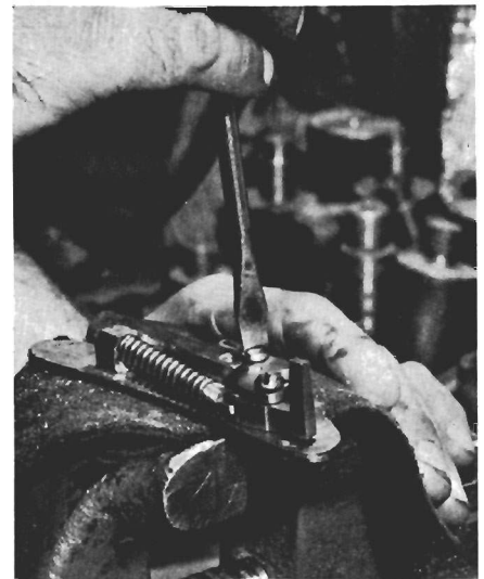
Hicks' lock design replaces old, fragile flat spring with durable wire coil.
