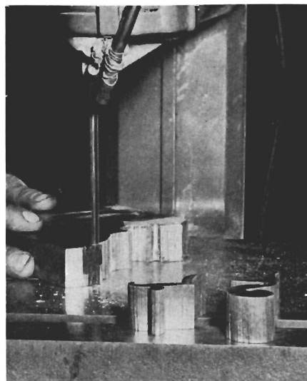
Hammer and frizzen are jig-sawed from steel plate and filed to shape.
