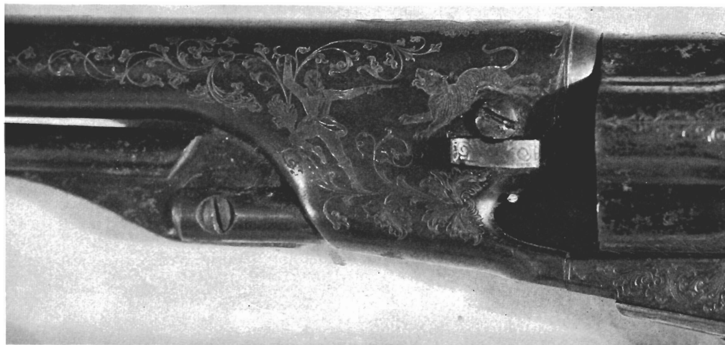
Delicate engraving on Colt New Police Pistol (shown about four times natural size) is very shallow. No abrasive cloth should ever be used to clean such guns, but only a little fine steel wool with oil.
