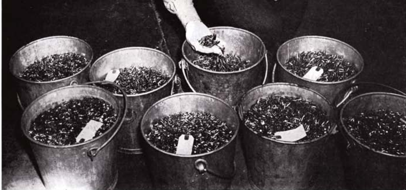
Each bucket of Sierra bullets, tagged by caliber and type, weighs about 170 pounds and holds about 8,000 missiles. Lead-point hunting slugs may become damaged through handling in plant, so visual inspection follows to cull out imperfect ones.
