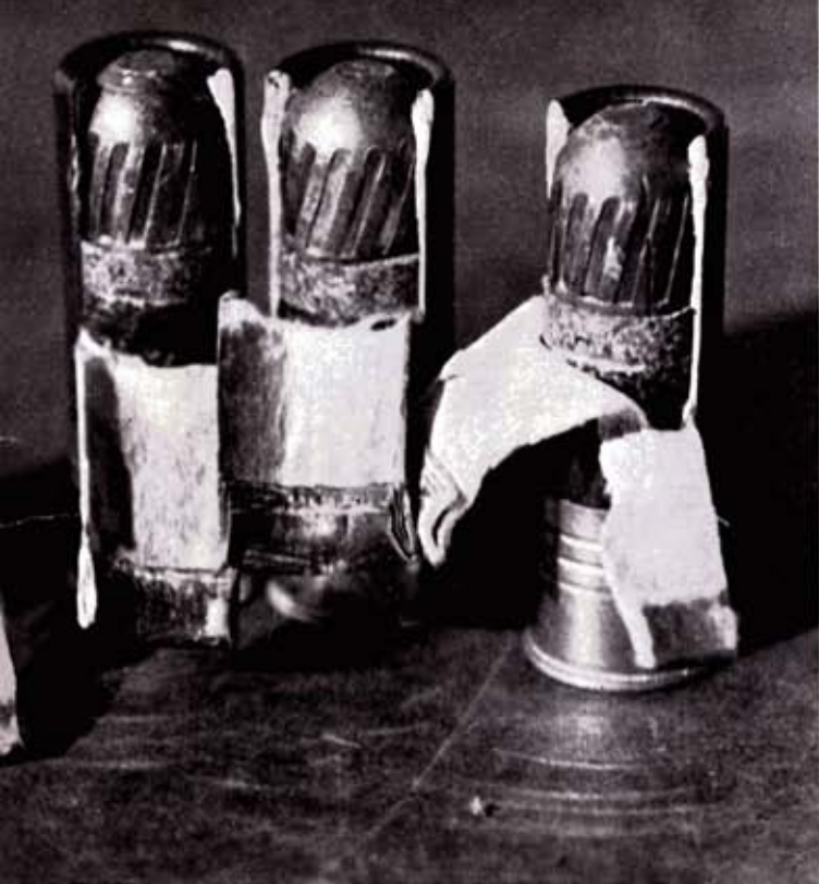
Slugs are sold in 12, 16, and 20 gauges in most makes like these high-base Federal loads. Rifle grooves are swaged on surface, are claimed to make ball spin in air.
