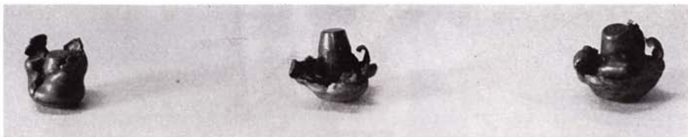
One-shot kills with Sierra bullets reveal hunting slug controlled expansion due to jacket thickness design. The 117-grain .257 boattail (left) took a 280-pound mule deer at 175 yards. The 130-grain .270 (center) got 250-pound mountain sheep at 300 yards. The 180-grain .30 boattail (right) folded up perfectly deeply penetrating hind quarter of deer.
