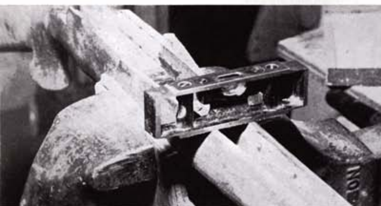
Bubble level is used to check stock edge and recoil block inside. Edges should be flat and perfectly horizontal.
