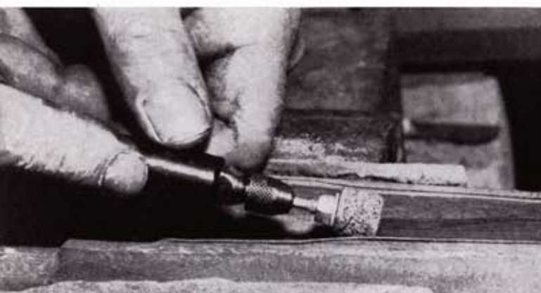
Rotary sander on flexible power cable can be used for rough-inletting barrel groove by routing between lines.
