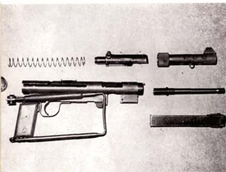
Swedish folding-stock gun is made from simple lathe-turned parts and tubing or cheap sheet-metal stampings.
