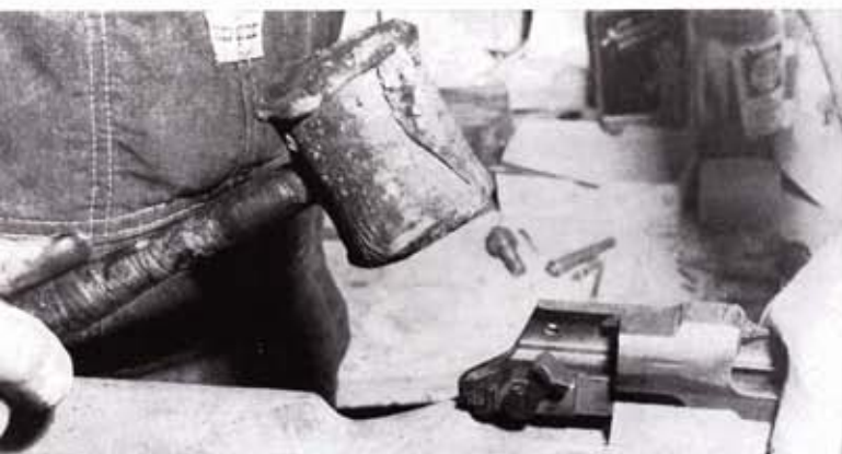
Tapping action tang with maul will mark wood where the lampblack touches, indicating contact spots to cut out.
