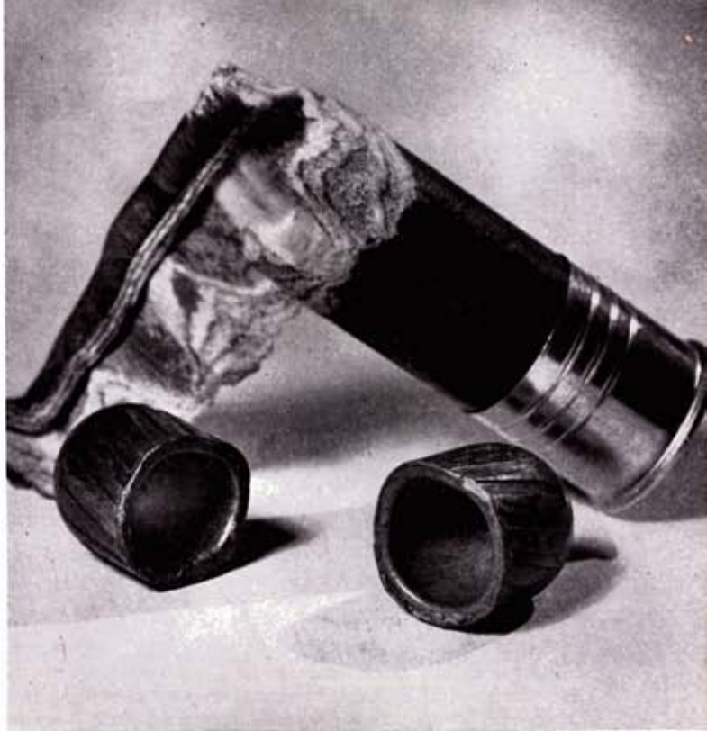
Thin skirts of slugs are dented in factory handling, and often distortion will contribute to smoothbore inaccuracy. Most slugs are undersized, a "rattling fit" in barrels.
