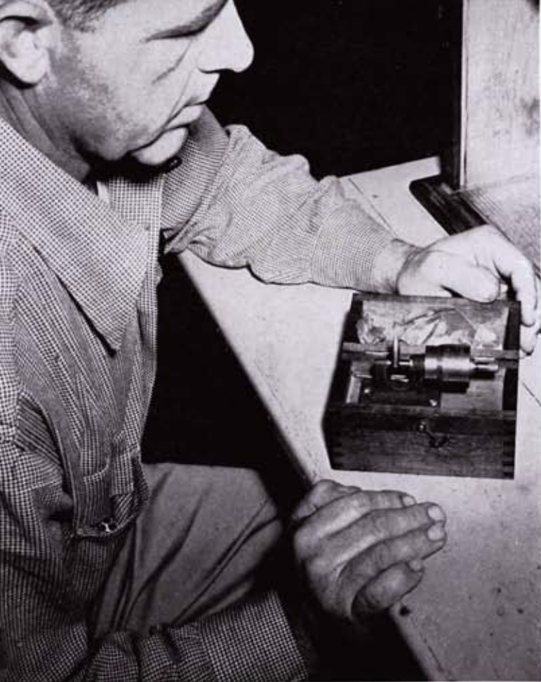
Micrometer measures slug diameter in frequent inspection checks during production to insure accuracy of bullet.
