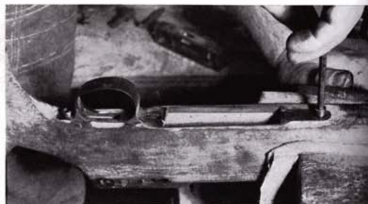
Allen screws are used in drawing guard plate snugly into stock. Screws are quickly removed and heads will not burr.
