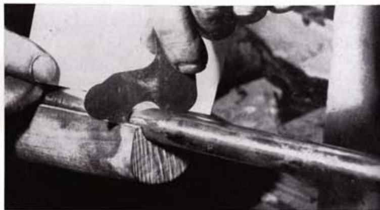
Template cut to diameter of barrel can be used to gauge depth of metal. Stock should almost come halfway.
