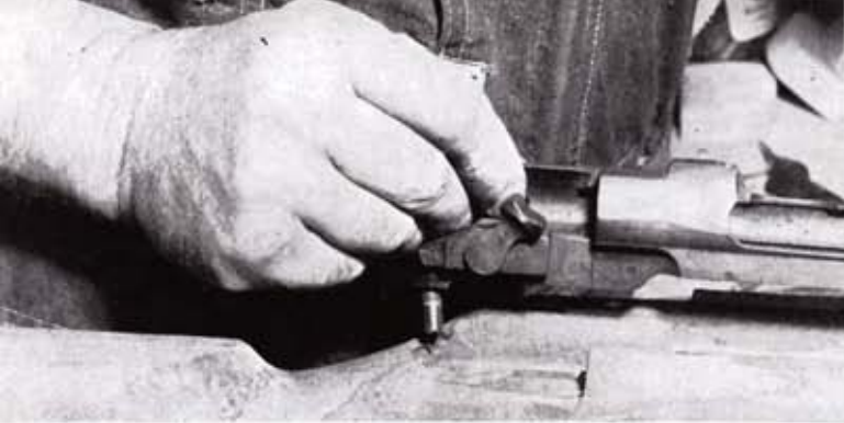
Enfield action which has been painted with lampblack is guided while inletting by headless tang work screw.
