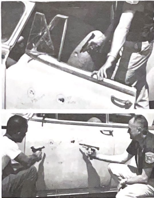
Practical police tests by G&A Handgun Editor Jeff Cooper (right) and handgun veteran Jim Sullivan on automobile bodies, comparing penetration of the .45 Auto and 9mm Luger, leaves little doubt as to the superiority of the big .45. Note how standard 230-grain .45 bullets penetrated door and upholstery. The Luger was erratic.
