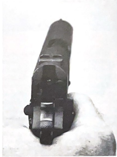
The .45 Auto has a narrower, slab-sided shape with a muzzle-heavy distribution of weight. It does not have the natural pointing qualities of better-balanced Luger.
