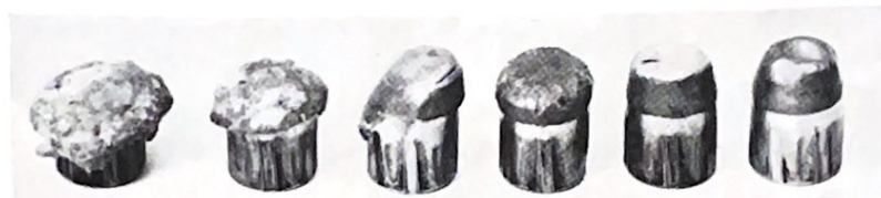
With the right bullets, the .45 Auto becomes a potent field gun. This is a lineup of bullets developed by bullet maker Mason Williams and fired into sand, clay and pine boards. Bullets are half-jacketed, soft lead with a shallow cup point — note expansion.
