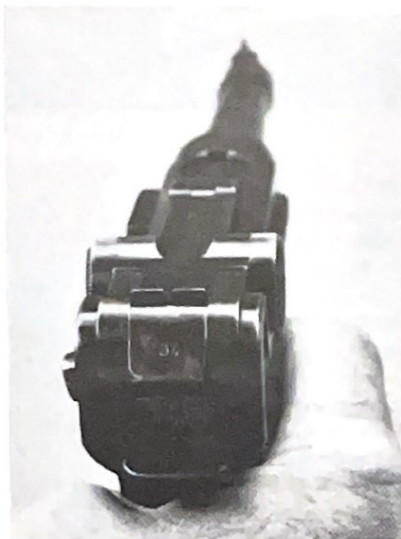
The Luger is famed for its superb balance and "pointing" qualities. Most of the weight is centered directly over the hand making the pistol distinctly muzzle-light.
