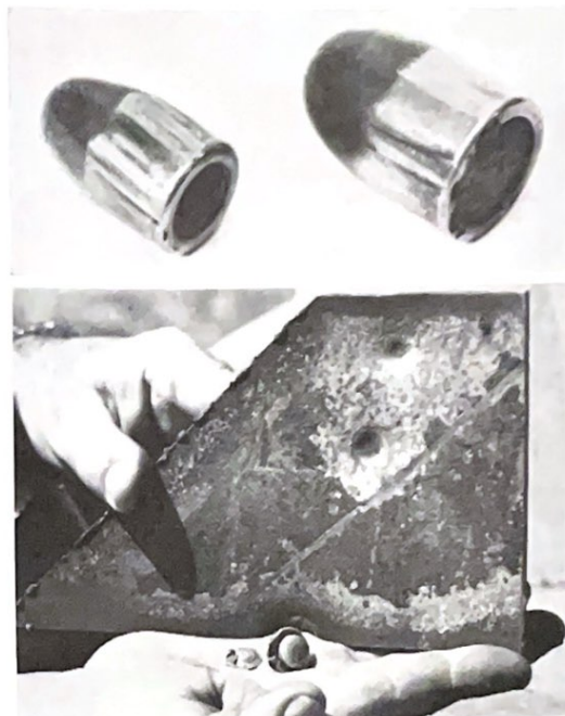
The difference between the 124-gr. 9mm bullet and the 230-gr. .45 Auto is apparent (top). Despite the 9mm's 1120 fps muzzle velocity, as compared with 850 fps for the .45, the latter carries a far greater punch as indicated by impact results on a 1/4-in. steel plate. Compare the bullets after the test — quite an eyeopener!
