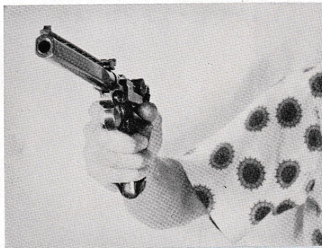
Slab-sided .45 barrel gives added mass, softens shock of big caliber recoil. Thumb-rest grips on new match pistol aid shooting. Left, shots load in fixed magazine.
