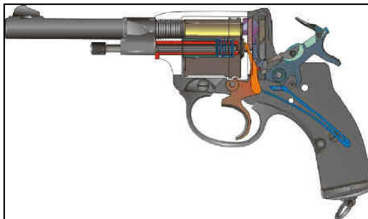
Cut-out view of the M1895 Nagant revolver
