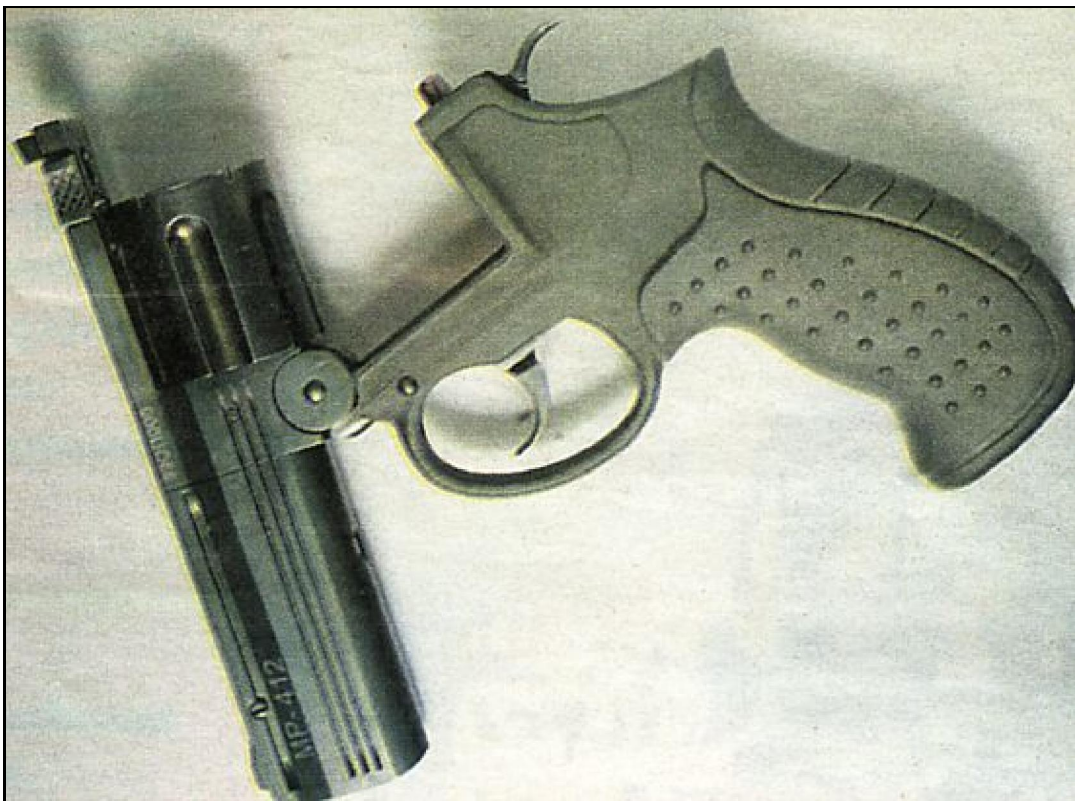
MP-412 Rex revolver, with barrel tipped down for reloading
