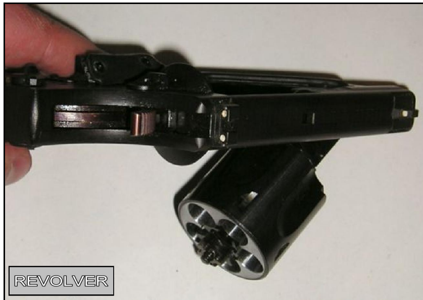
OTs-38 revolver, top view with cylinder opened for reloading. Note the most unusual way of cylinder opening.
