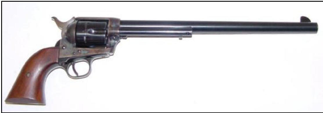
Colt 1873 Single Action Army, Buntline Special model with 12 inch barrel.
