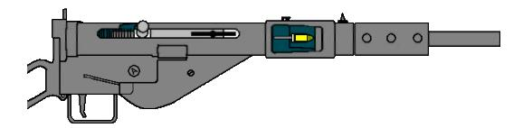
The Sten was an incredibly simple weapon that utilized the system known as 'blowback'. The diagram above gives an idea of how the Mk.II Sten fired 3 rounds on automatic, only much slower than in reality - in one second, the Mk.II firing at a rate of 540 rpm, could fire nine rounds. A basic description of the operation of the system is as follows:
