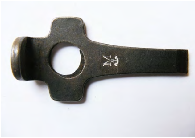
Two Reichsmarine (German Navy) variations: these are in the white, and the sides are not smoothed with a file.
