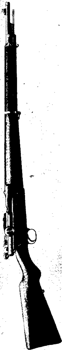
MODEL 98. MAUSER SEMI-AUTOMATIC RIFLE WITH CLAW BLOCK LOCK. SHORT RECOIL SYSTEM.
