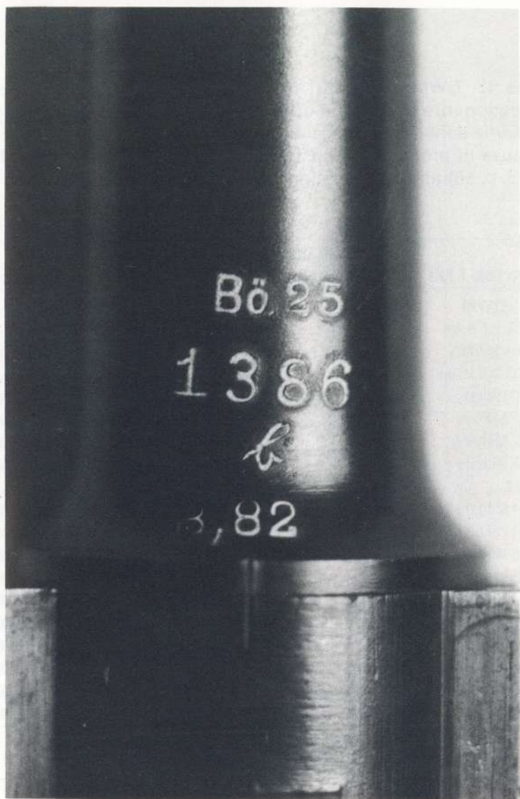
Figure 6e. The Bö 25 stamp on this 1913 DWN indicates the barrel is made of Böhler steel. This stamp is found on a very few 1913 and 1914 DWM and Erfurt Lugers. It indicates hardness for an experimental hardness process.
