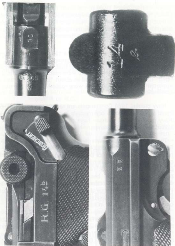
Figure 7 1908 DWM commercial military (s.n. 60530) Luger with double Crown/B military stamps on the receiver, 8.83 military barrel land diameter on the barrel, R.G. 14 b engraved on left side panel before blueing and 14 b stamped on magazine. The R.G. is the designation for the Reichs Gendarmerie, a paramilitary police force that was active in the Alsace Lorraine and the colonies prior to 1918. It likely had close ties to the Imperial military. See figure 25. Pistol and photograph from the collection of D.J. Rousseau, Anchorage, Alaska.
