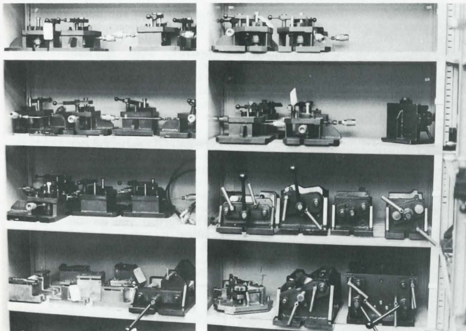
A small portion of the quarter-million dollars worth of jigs and fixtures that Mauser built and had built from scratch for the Parabellum. All this just to hold the parts in the machines.
