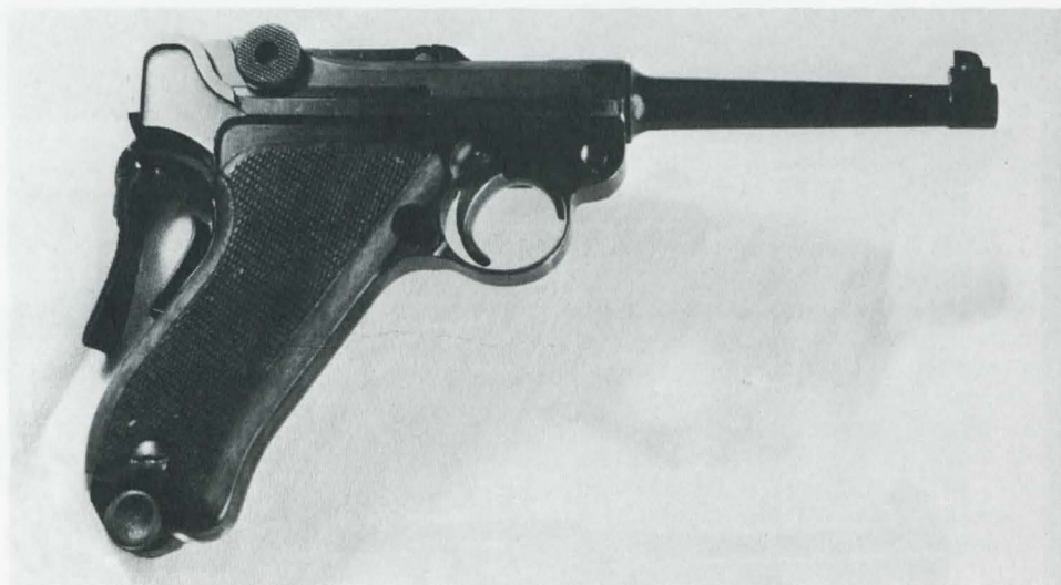
Controversial Model 1924 Swiss is easily recognisable by its flatsided grips, dull finish, and "Waffenfabrik Bern" inscription on the front link. Despite the label, it probably went into production in 1913.
