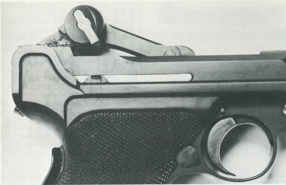
Weaknesses, both for production and in use, led to modifications all through Parabellum history. Above, it took a toggle lock and frame hook to hold the delicate beast closed in early models. To keep trash out of the trigger linkage, the Germans made the intricate sideplate at left below; this cost the Swiss too much, so they sliced straight across (at right). The latter plate is the one to be on the new Parabellum. Eventually, the Germans couldn't stand the gaff, dumped the Luger and went for the P-38 (bottom), a much better combat pistol.
