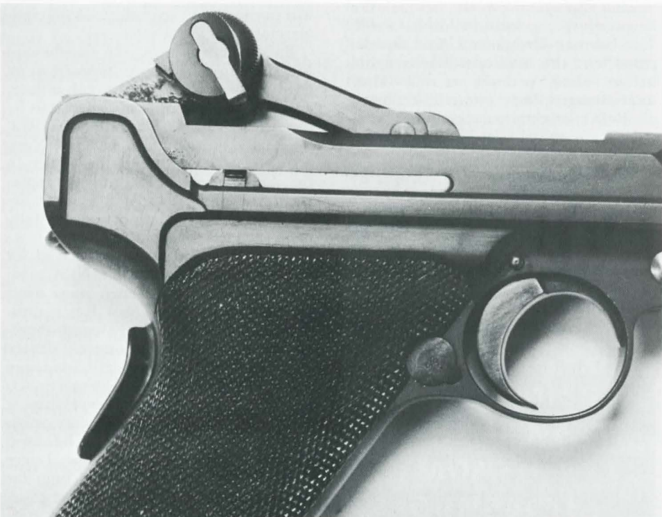
Close-up shows toggle lock ready to pounce down on frame hook, providing it makes it. This was the model first adopted by Switzerland in 1901.
