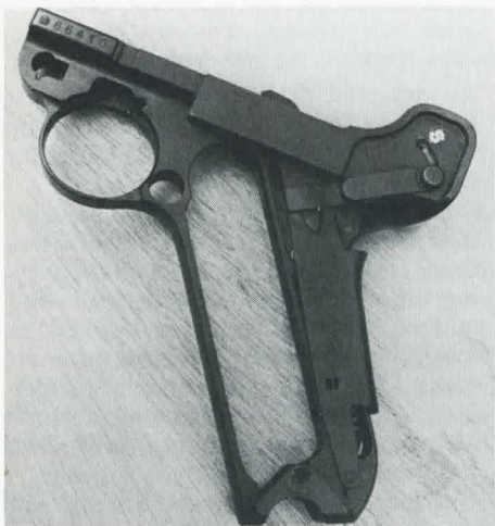
Grip safety on M29 was stamped, a sensible move. Only function of thumb safety is to block grip safety, and a stamping works just fine for this.
