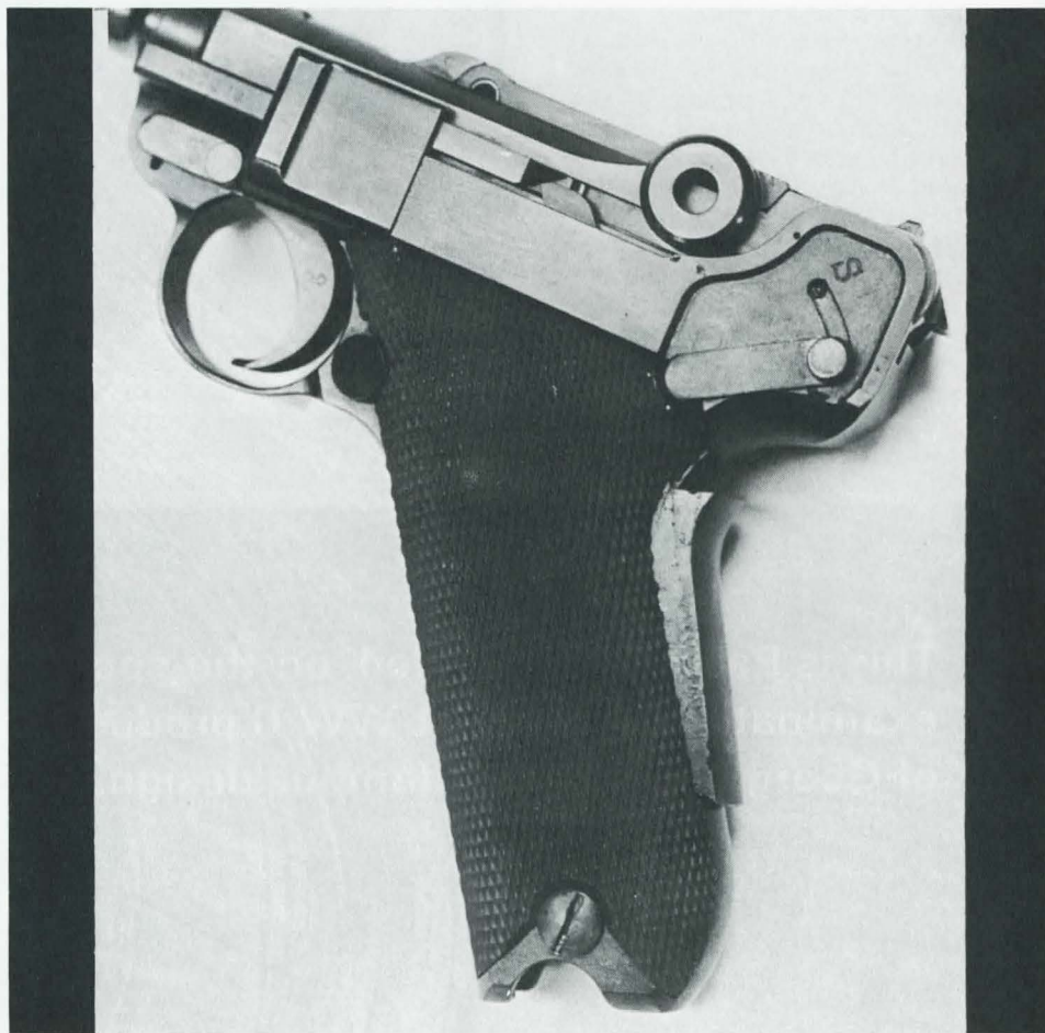
The 1929 Swiss, replete with tool marks and red plastic handle, is no thing of beauty, and that, says Stevenson, was the Luger's prime purpose. Note straight front strap, flat safety, and total absence of knurling
