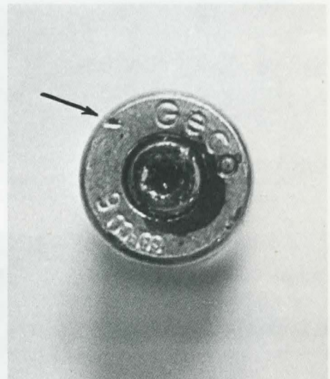
4-o'clock ejector imprint shows clearly on soft Geco brass. Case mouth is fated to be bashed in on the opposite side.
