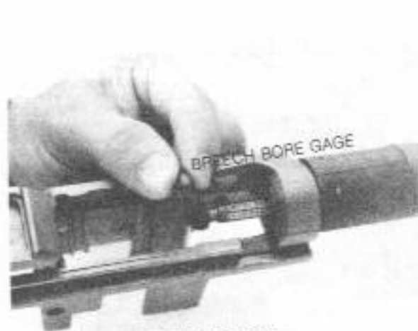
Figure 50. Gaging breech bore.
