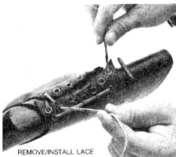
Figure 56. Installation/removal of cheek pad assembly, Rifles M 1C and M 1D (Sniper's)
