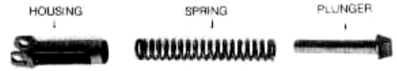
DISASSEMBLE/ASSEMBLE HAMMER SPRING HOUSING, HAMMER HELICAL COMPRESSION SPRING AND HAMMER SPRING PLUNGER
