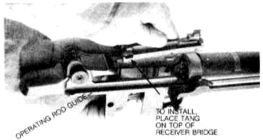
Figure 19. Disassembly / assembly of trigger housing assembly (4 of 4).
