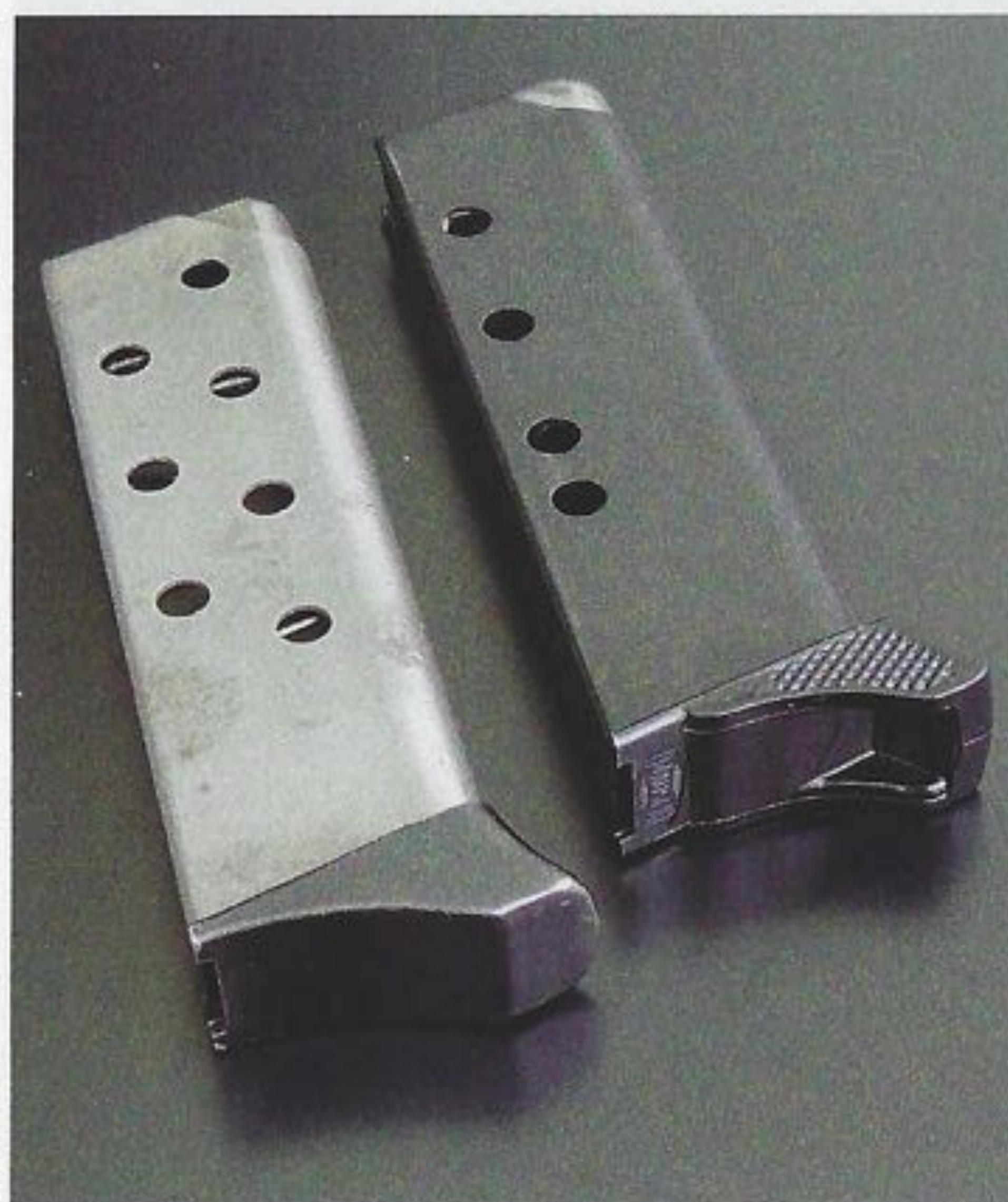
The magazine from wartime production is not blued and has a finger extension made of metal, while for the blued magazine of the postwar production the finger extension is made of plastic.
