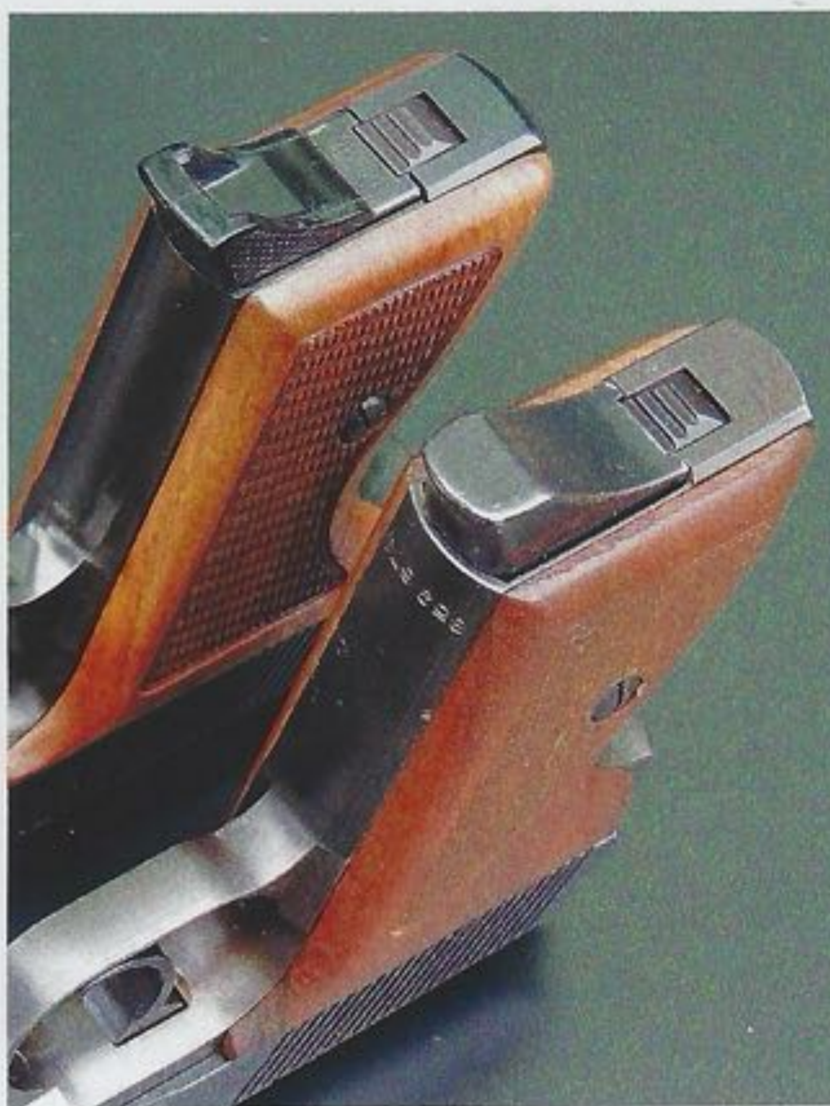
The magazine from wartime production is not blued and has a finger extension made of metal, while for the blued magazine of the postwar production the finger extension is made of plastic.
