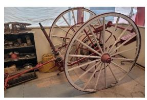
Prior to **1939** fires were fought with a hose cart and 30-gallon fire extinguisher on two wooden wheels. The fire extinguisher had a short hose and a pump, but it was too large to get into a structure. Water was supplied by only a 70 ft. water tower with only 31 lbs. of pressure. They were stored in the back of the old jail house, currently the Wilder Museum.
