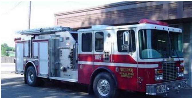
In 2003 the Fire District purchased its first apparatus with the specific purpose of fighting brush / grass fires. It was constructed by mounting a 2003 GMC 2500HD Duramax Diesel pickup and a 250-gallon poly tank skid unit the bed. This was a fast attack/off-road truck but had a very limited water supply. This was partially offset with the addition of a foam injection unit that amplified the extinguishing properties of the water.
