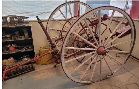
Prior to **1939** fires were fought with a hose cart and 30-gallon fire extinguisher on two wooden wheels. The fire extinguisher had a short hose and a pump, but it was too large to get into a structure. Water was supplied by only a 70 ft. water tower with only 31 lbs. of pressure. They were stored in the back of the old jail house, currently the Wilder Museum.
