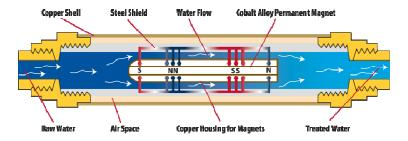
Con-Serv Manufacturing has been installing physical conditioners on the Eliminator Series of Spot Free Rinse Systems for years. As a pre-treatment for RO systems, the precipitated suspended solids will be discharged to waste along with dissolved solids, rather than plating out on the membrane surface. In addition, the Physical Water Conditioner reduces surface tension of water, increasing its wetness or penetrability.
