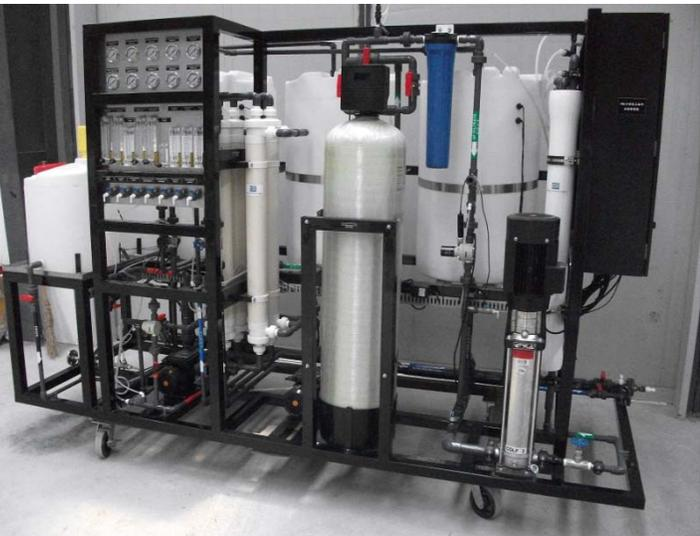
Shown: UF(8 gpm)/ Spot Free Rinse System (3 gpm)
