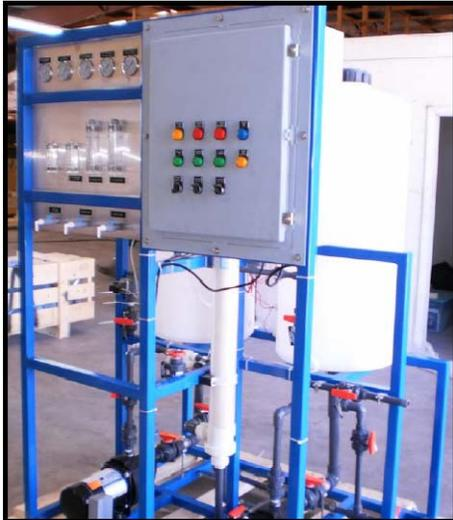
Shown: UF system 4 gpm
