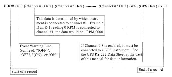
If an error occurs on any channel due to a problem in an instrument or data line, "ERROR CH1", "ERROR CH3", etc. will be placed in the record, indicating on which channel the error occurred.
