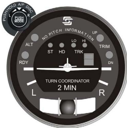
Fig. 2-4. AP Display, Turn Coordinator Failure (System Twenty)
