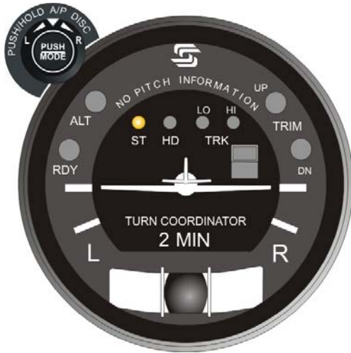
Fig. 2-17. AP Display, ST Mode Engaged (System Twenty)
