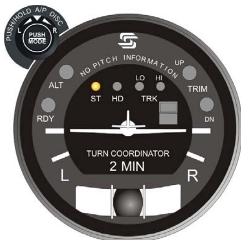
Fig. 2-21. AP Display, ST Mode Engaged (System Thirty)
