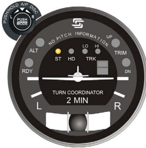
Fig. 3-1. AP Display, ST Mode Engaged
