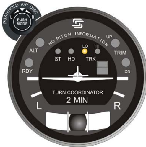
Fig. 3-3. AP Display, LO TRK Mode Engaged
