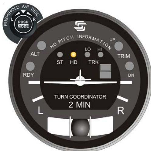
Fig. 2-22. AP Display, HD Mode Engaged (System Thirty)
