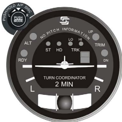
Fig. 2-9. AP Display, All Lamps Extinguished (System Thirty)
