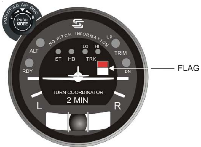
Fig. 2-12. AP Display, Low Voltage Flag (System Thirty)
