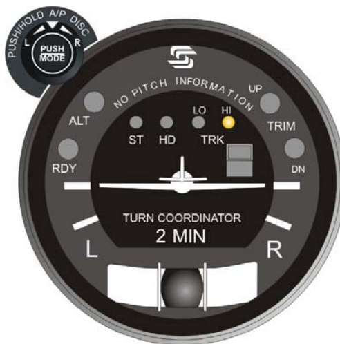
Fig. 3-4. AP Display, HI TRK Mode Engaged
