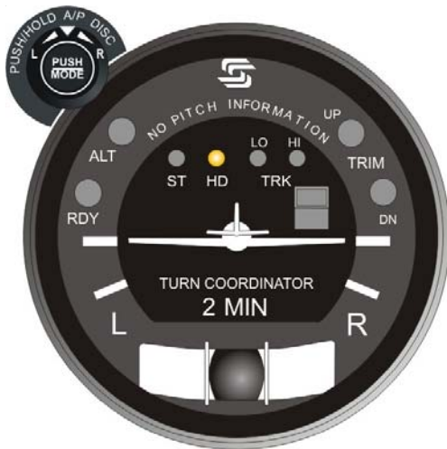
Fig. 2-18. AP Display, HD Mode Engaged (System Twenty)
