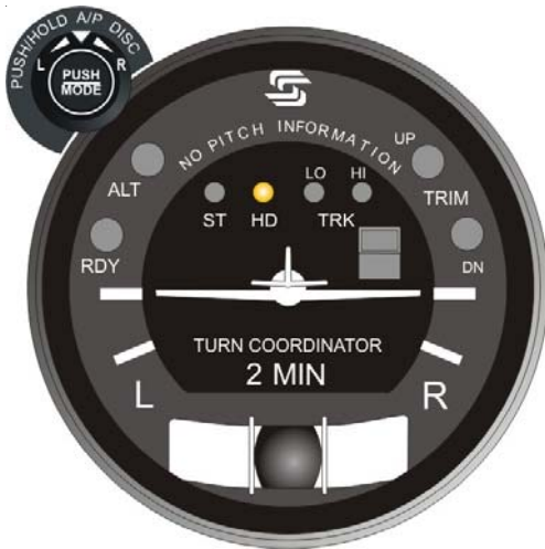
Fig. 3-2. AP Display, HD Mode Engaged
