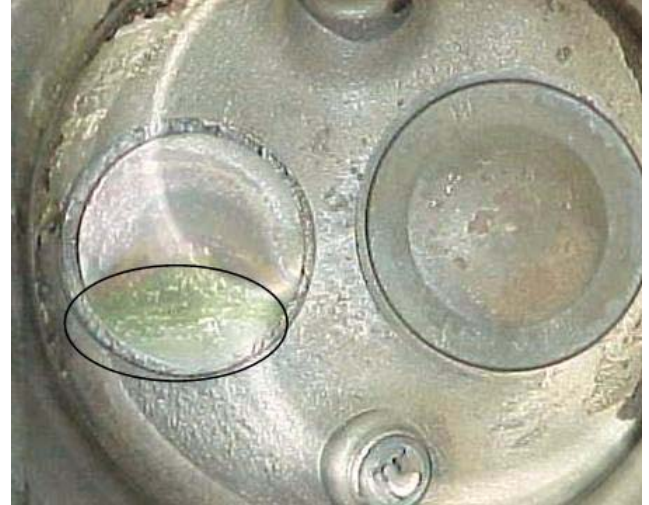
Burned Exhaust Valve
