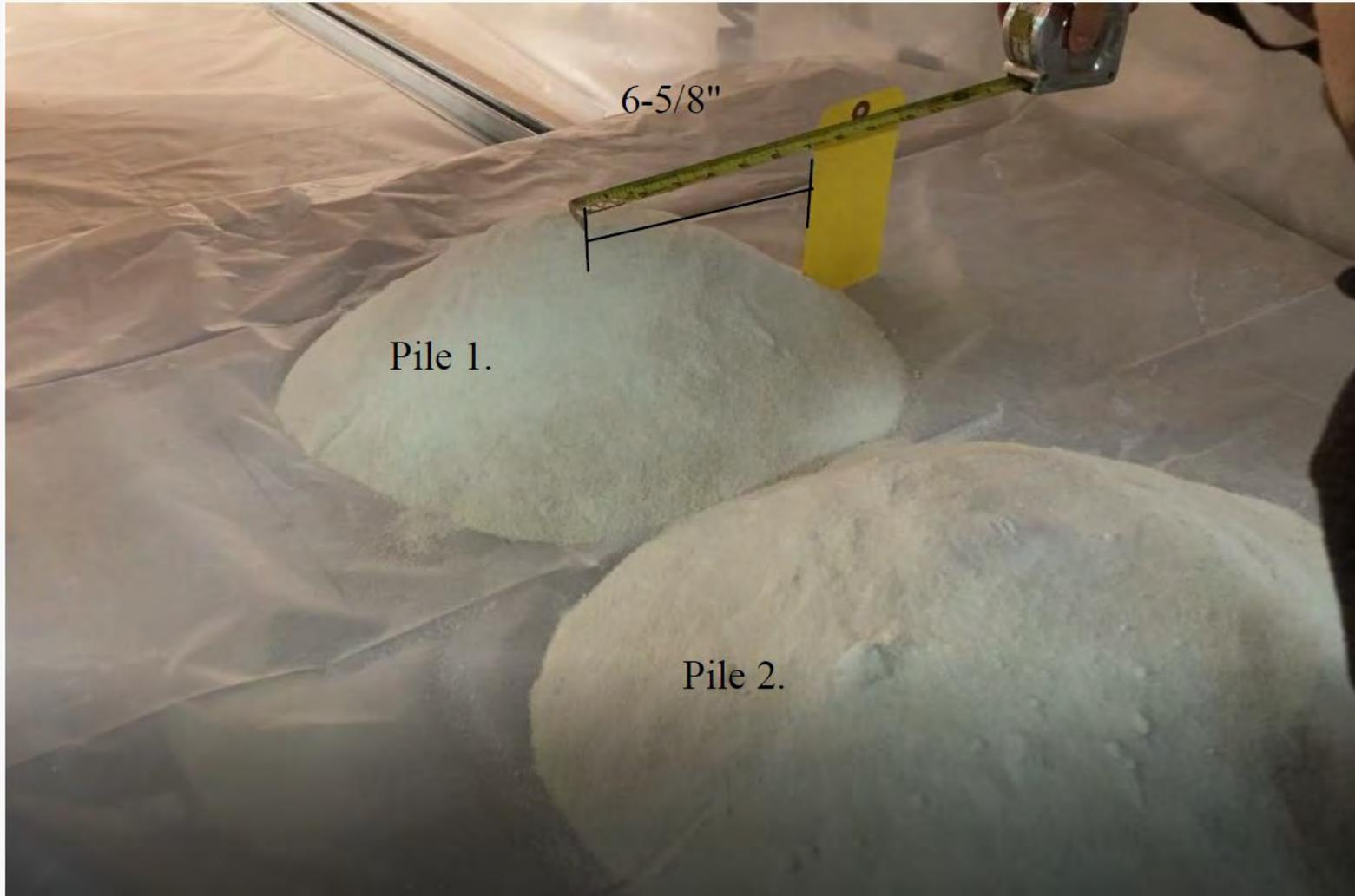
**Measurement taken from center line to 1" of depth**
