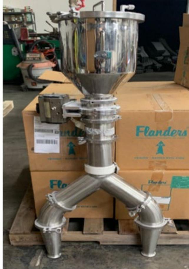
Hopper reduces in diameter from 4" to 2" at each nozzle
