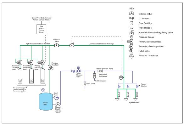
Fig. 1. Schematic of engineered hybrid fire extinguishing system
