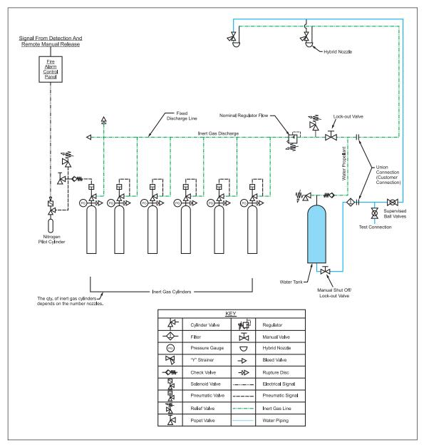
Fig. 2. Schematic of pre-engineered hybrid fire extinguishing system
