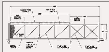
Chain Link Cantilever Gate (Detailed Example)
