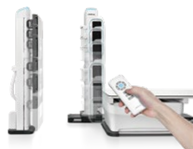
Bidirectional synchronization of the tube and bucky
