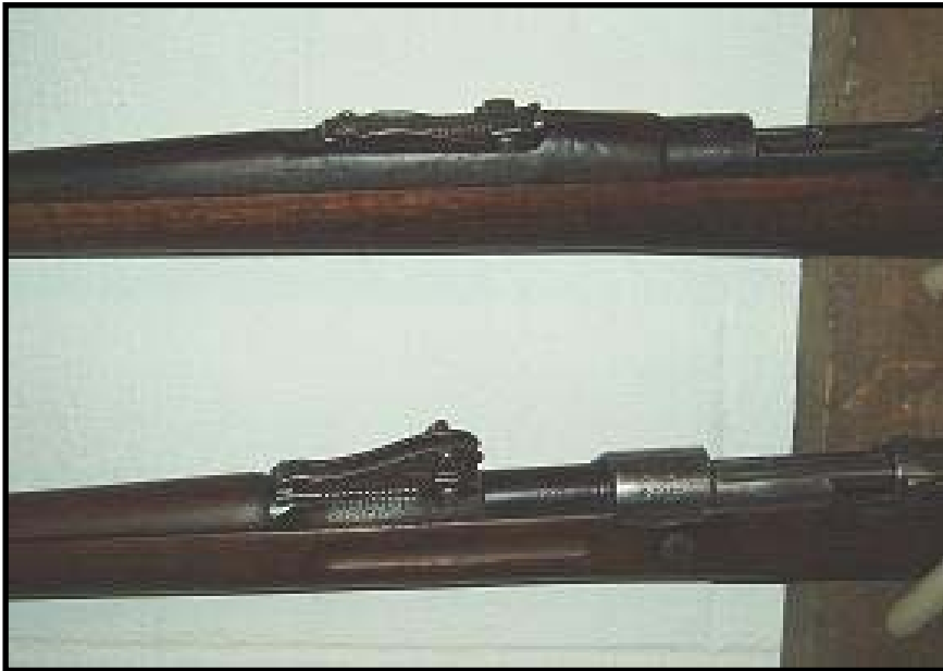
Fig. 1 Comparison of CZ 98/22 (top) to Gew. 98 (bottom). Note the differences in sight and hand guard.
