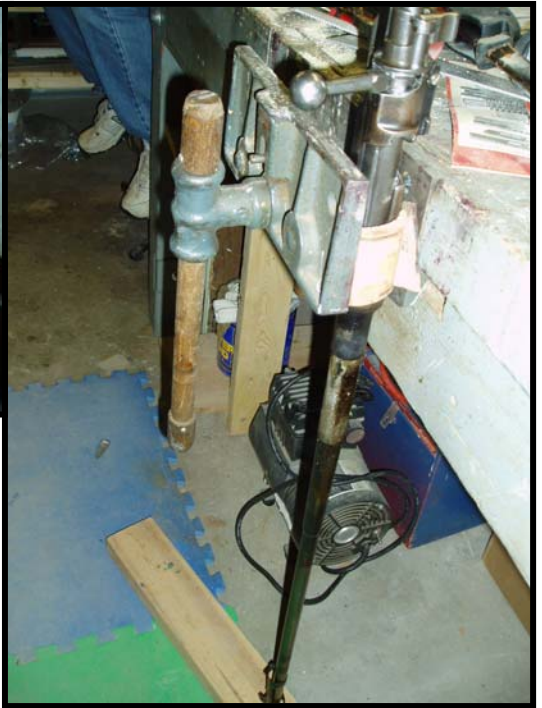
Fig 3. Using a propane torch, the barrel and sight are heated to loosen the solder. Be sure to heat the barrel evenly (above and below the sight) to prevent warping.
