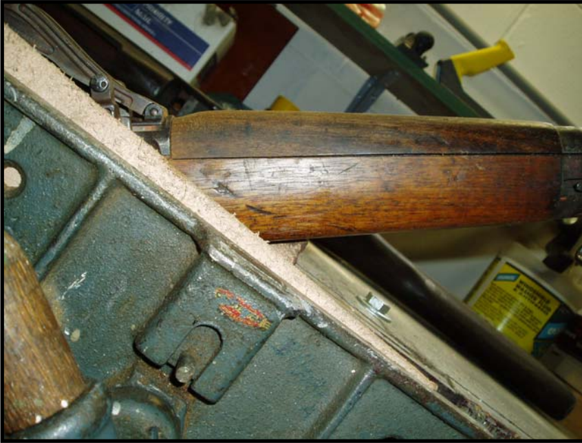
Fig. 15. Profile of guard after sanding. The angle of the 'slope' in front of the Lange sight is slightly more radical than the original.
