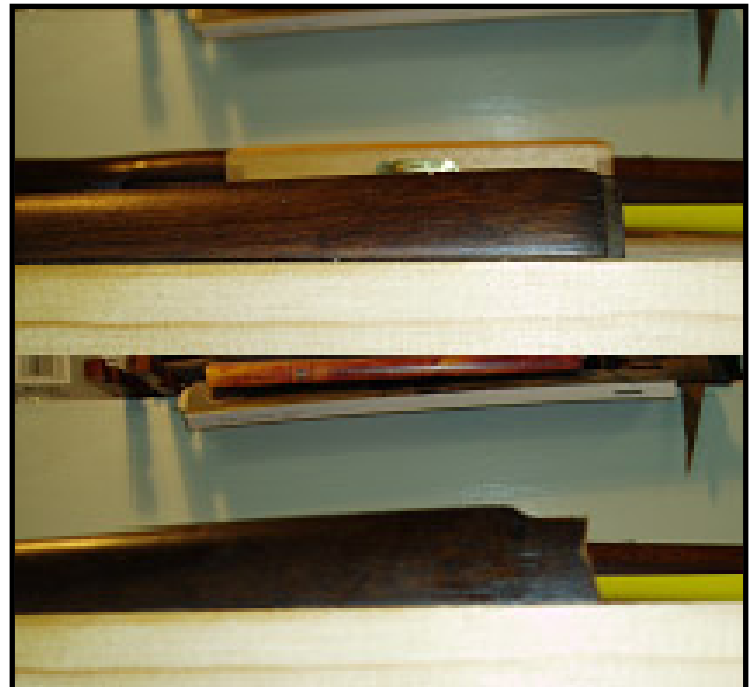
Fig. 11. The original hand guard profile (top) and the initial Cz98/22 profile (bottom)
