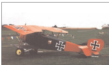
Marvin's plane is a Siemens-Schuckert D-1b, which differed from the D-1 in that it had a one-piece upper wing, one machine gun, and a spinner. Colors are of no particular pilot—Richthofen's color scheme was copied in orange. The bottom surfaces are in the standard German camo pattern.
