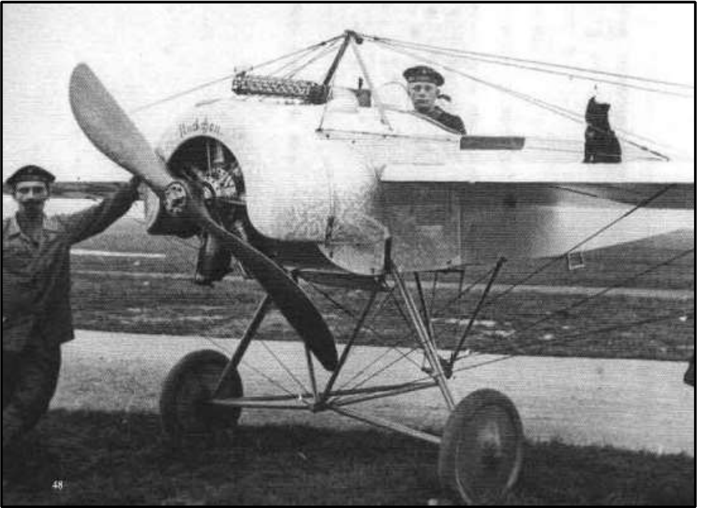
The first true fighter, the Fokker Eindecker E.I with a synchronized machine gun
